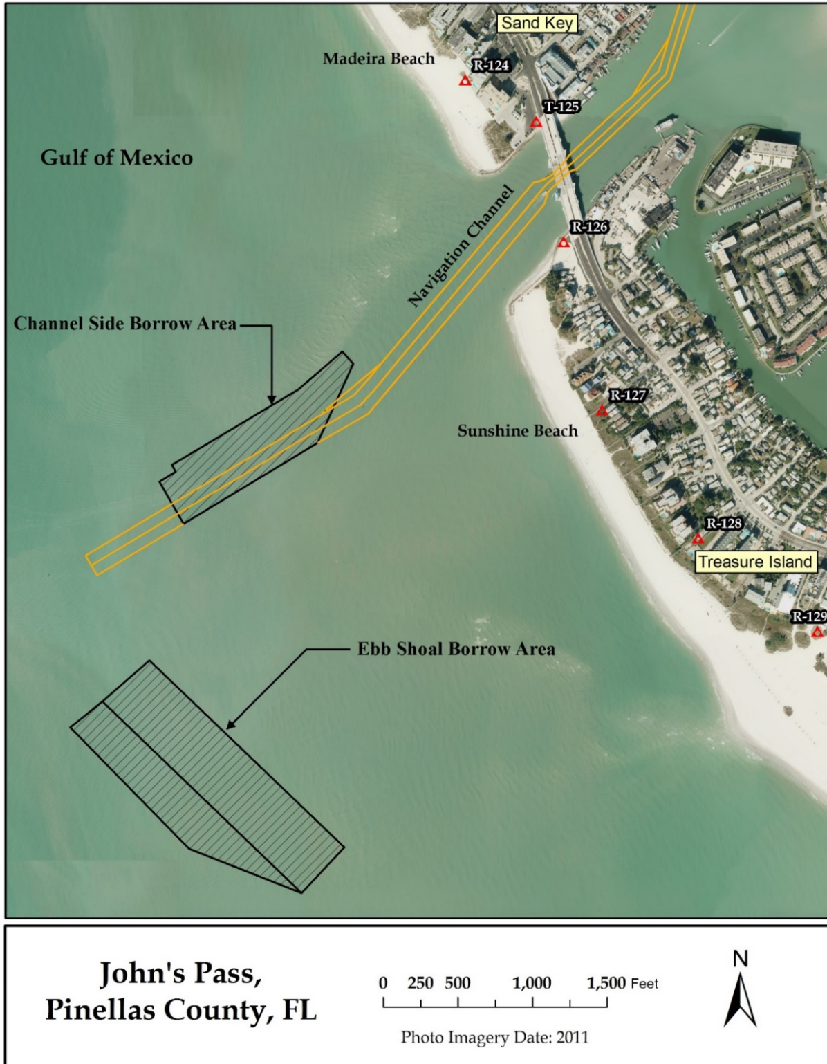
Figure 3. The authorized navigation channel, ebb shoal and channel side borrow areas for John's Pass. 2011 aerial photo courtesy of the SWFWMD.
