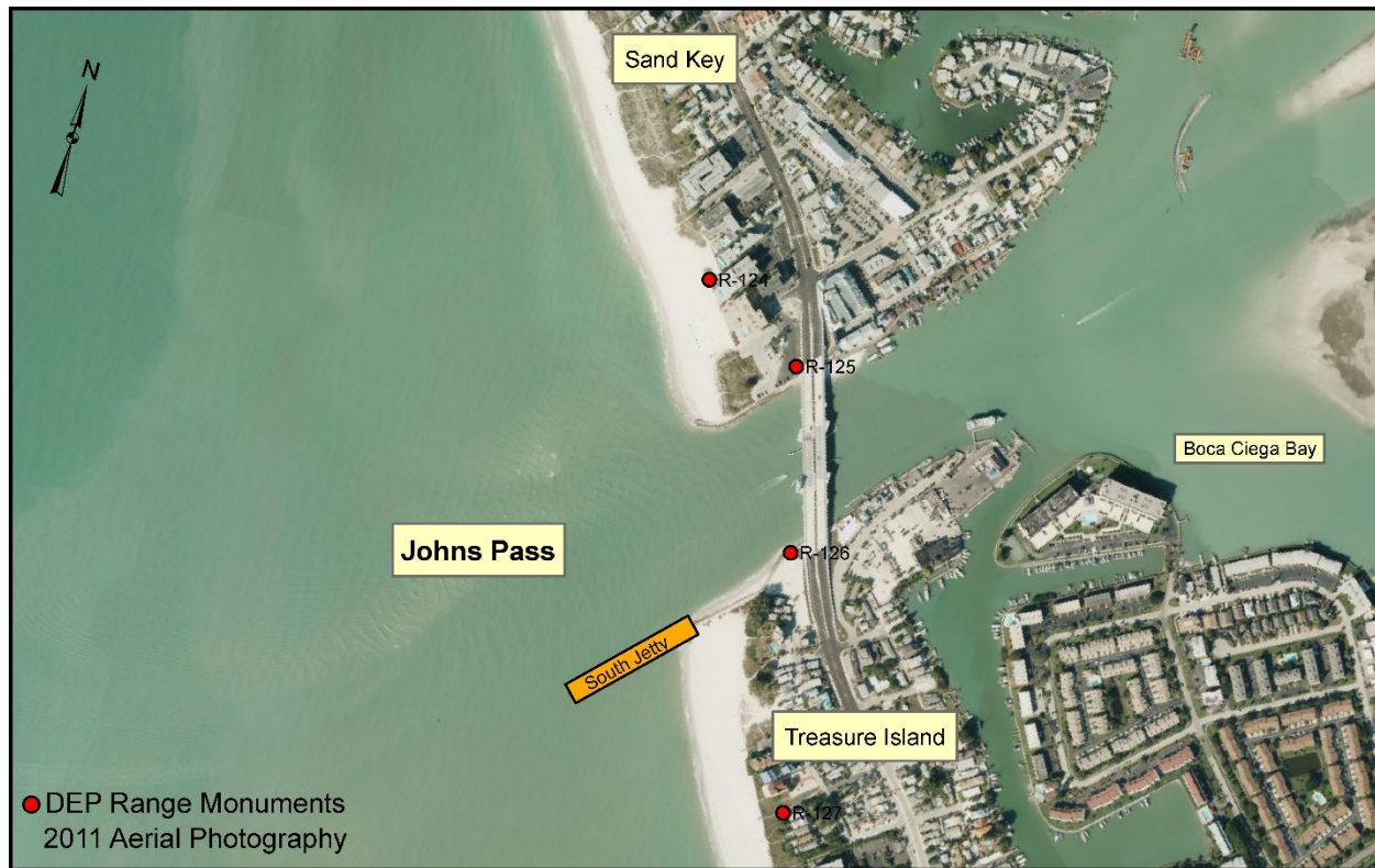
Figure 8. Alternative 5 illustrating an extension of the south jetty (Wang et al., 2016). The 2011 aerial photo is courtesy of the SWFWMD.
