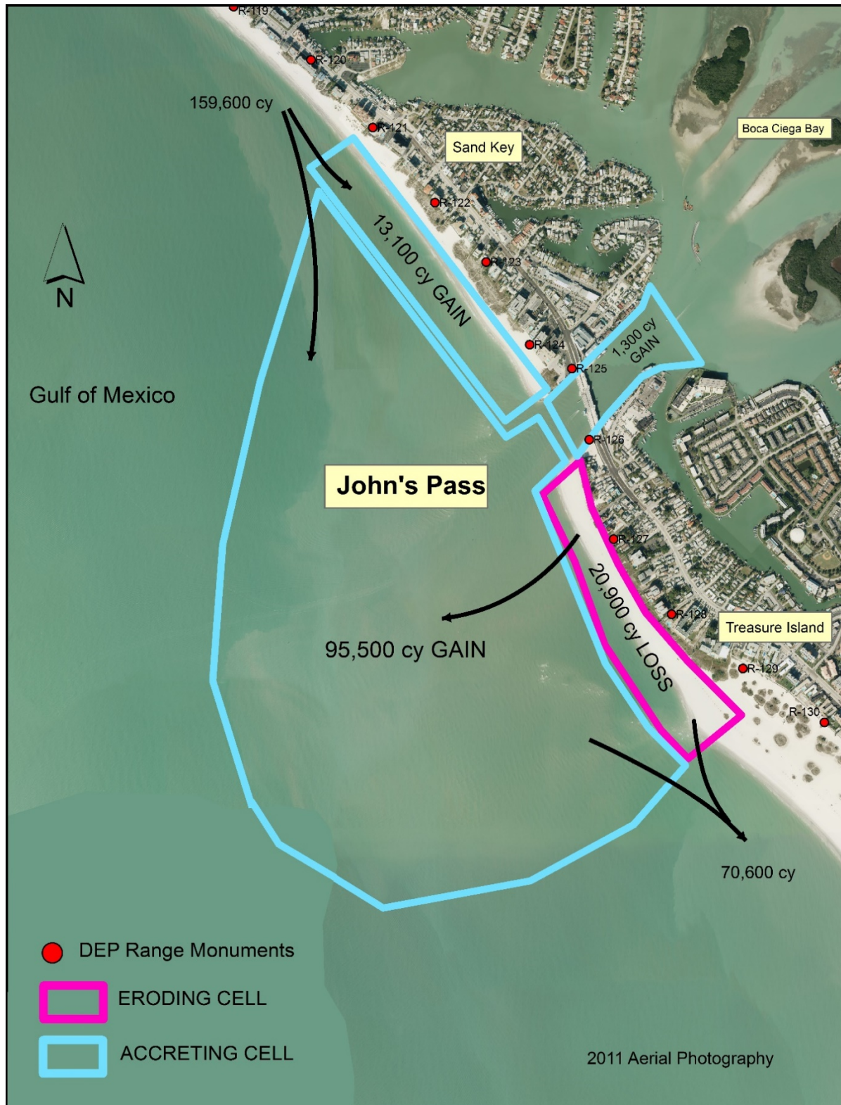
Figure 12. Annualized sediment budget at John's Pass determined based on field data collected from October 2010 to June 2014 (Wang et al., 2016). The 2011 aerial photo is courtesy of the SWFWMD.
