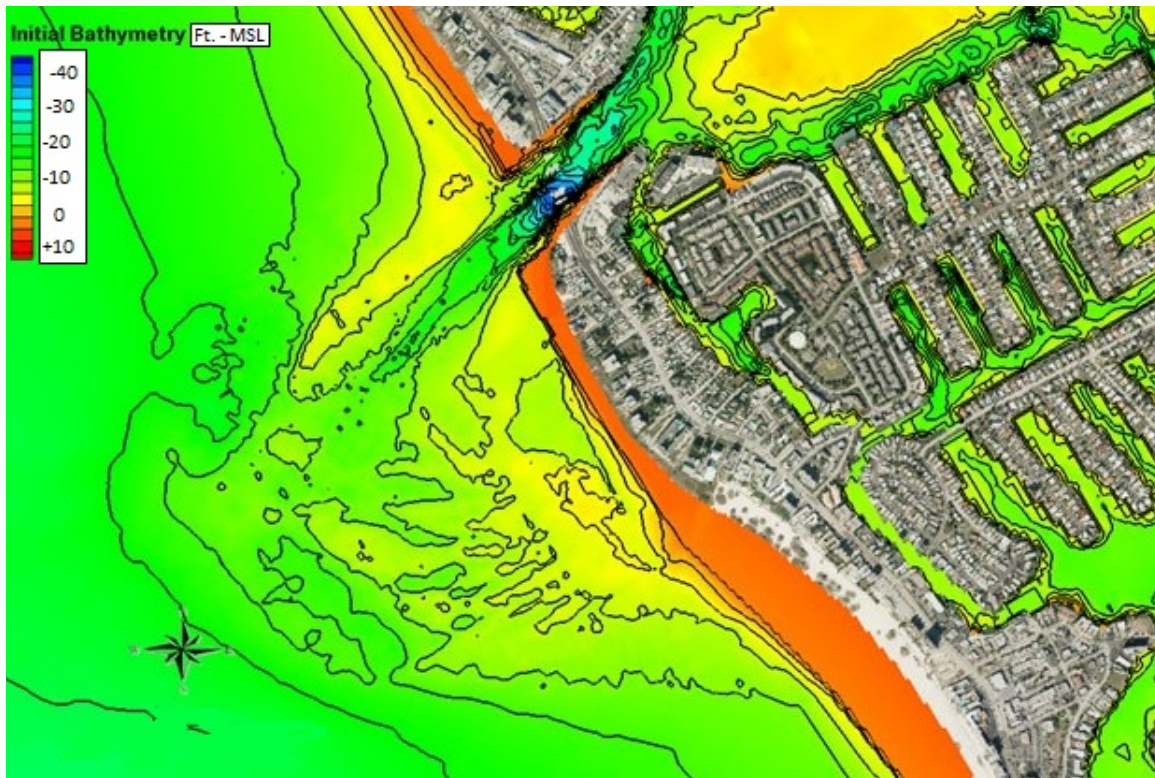
Figure 4. Initial bathymetry illustrating the present conditions at John's Pass (Wang et al., 2016).
