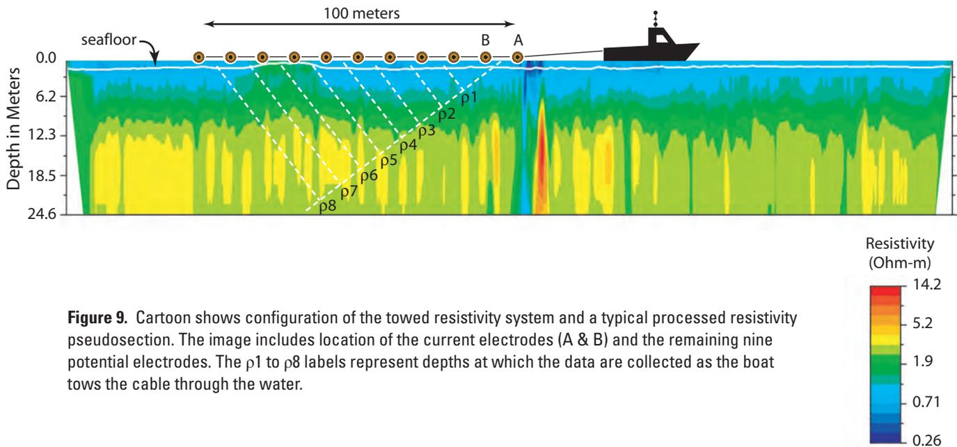
**Figure 9.** Cartoon shows configuration of the towed resistivity system and a typical processed resistivity pseudosection. The image includes location of the current electrodes (A & B) and the remaining nine potential electrodes. The  $\rho_1$  to  $\rho_8$  labels represent depths at which the data are collected as the boat tows the cable through the water.
