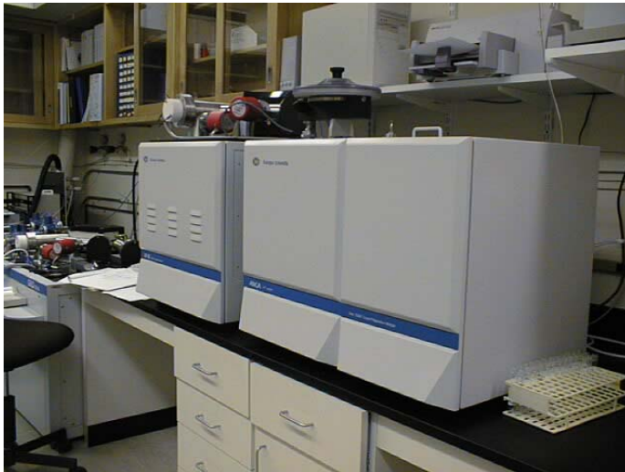
Figure 5: Elemental analyzer and stable isotope mass spectrometer utilized in this study.
