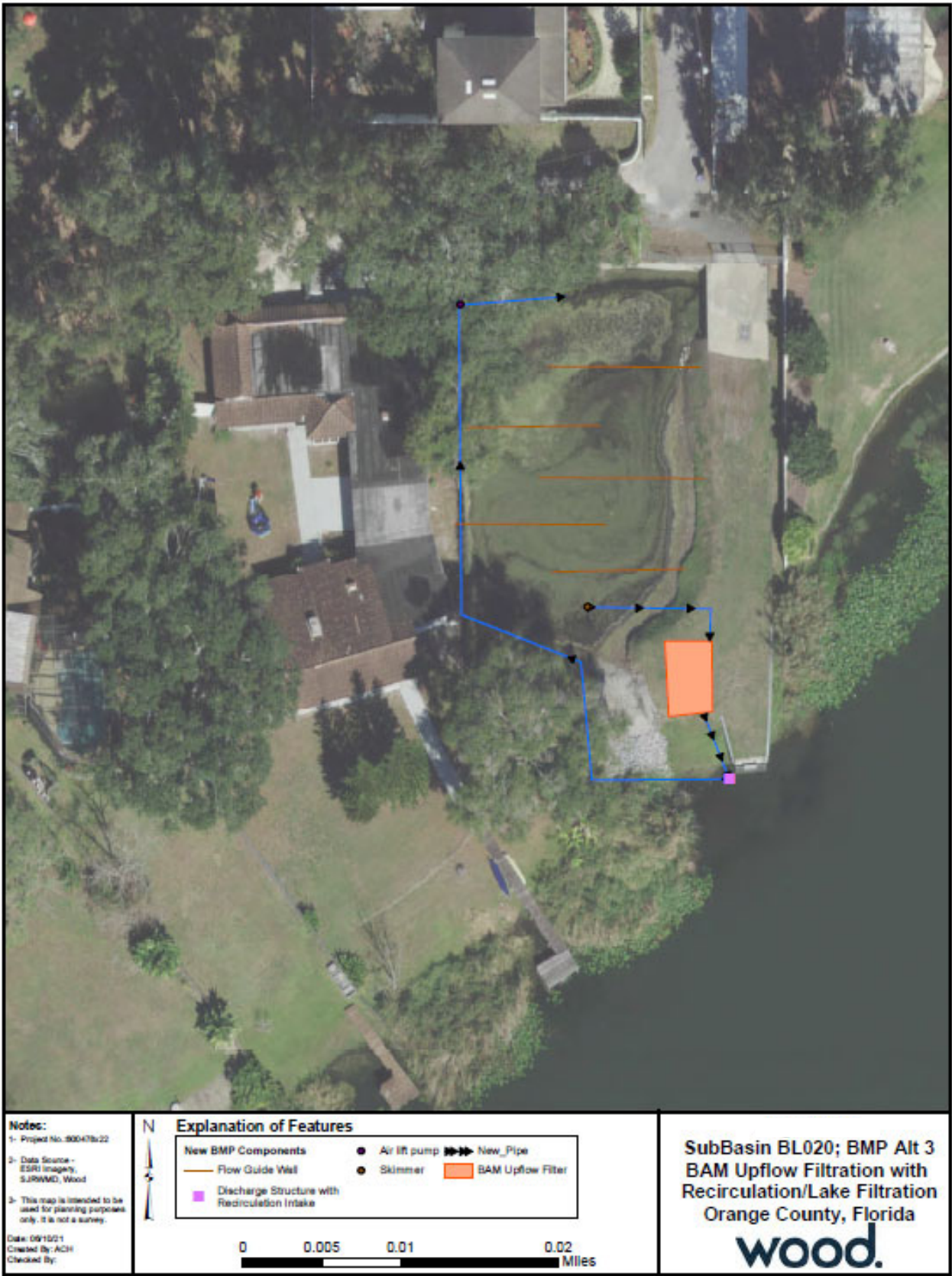
Figure 6: West BAM Upflow Filter
