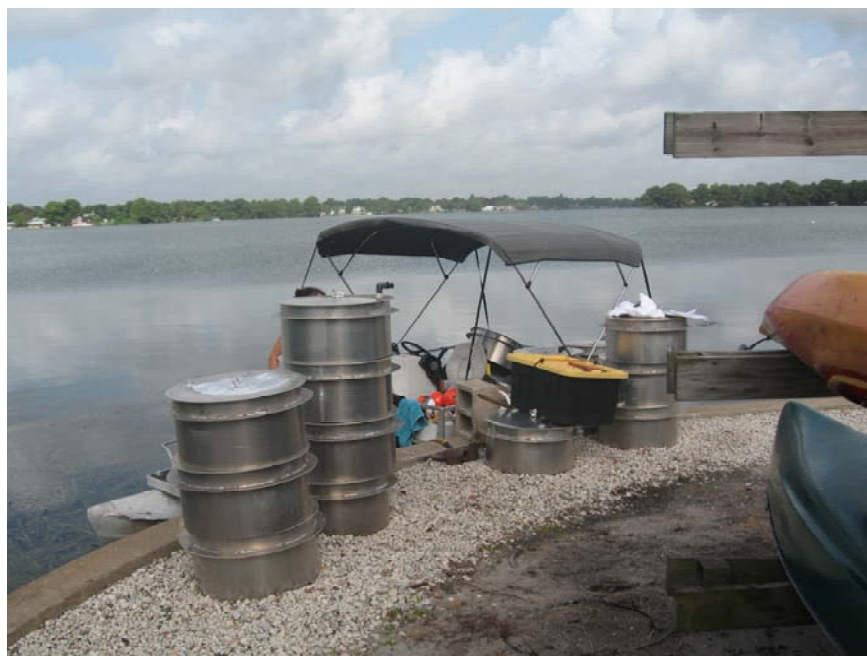
Figure 4-3. Seepage Meters Being Prepared for Installation.
