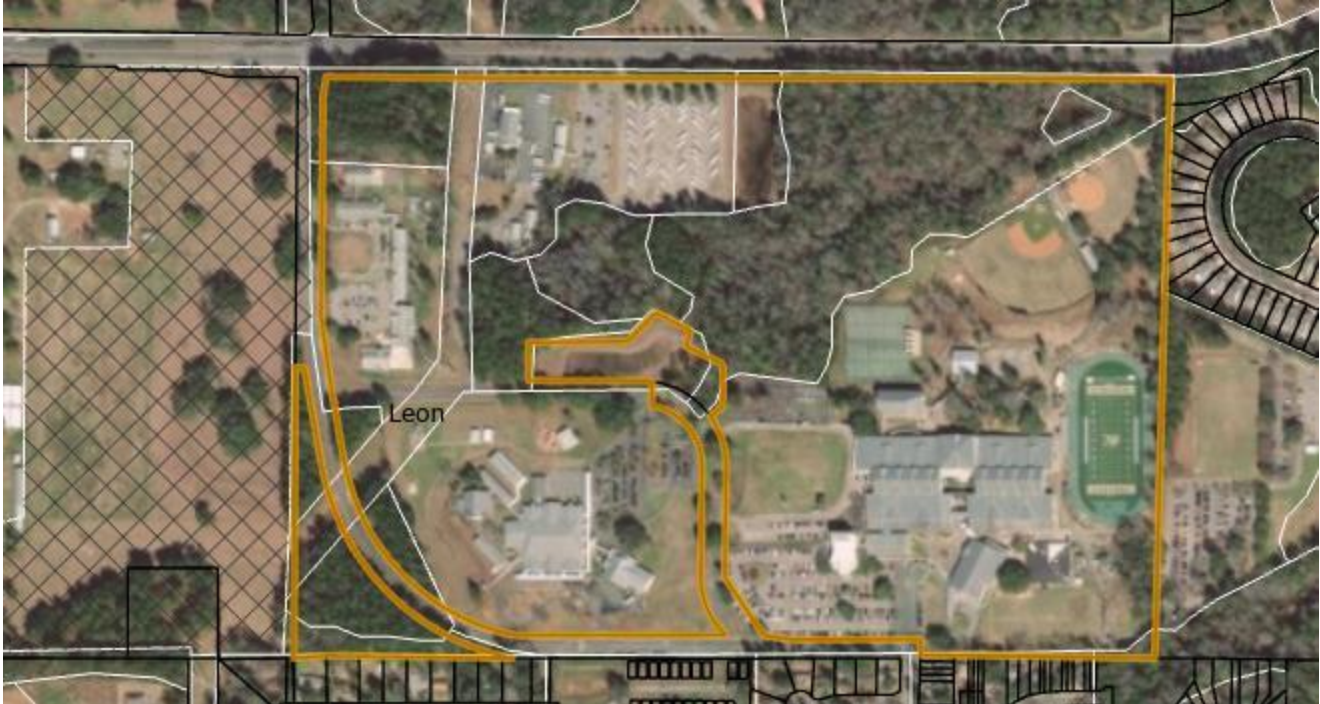
Figure 29. Multiple public school campuses on 1 DOR parcel feature. Orange outline feature is the parcel feature for this school complex. LULC features shown with white outline. Note: 4 LULC features represent separate campus and bus compound areas and also several features represent the wetland and forested areas on the school property.
