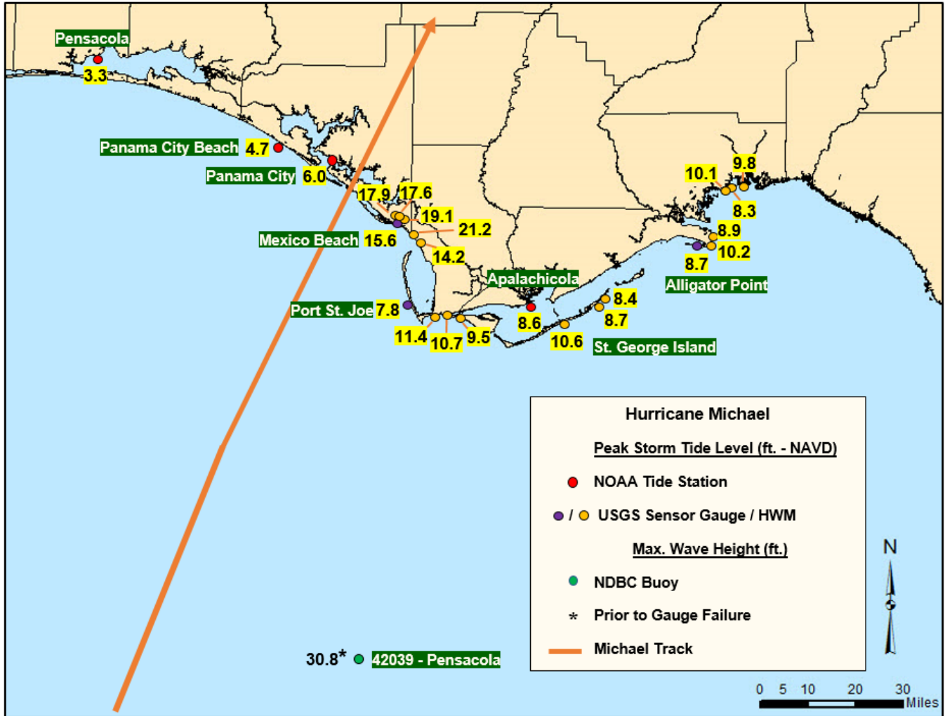
Figure 6. Hurricane Michael peak storm tide levels and the maximum offshore wave height [Data sources – NDBC, NOAA and USGS].
