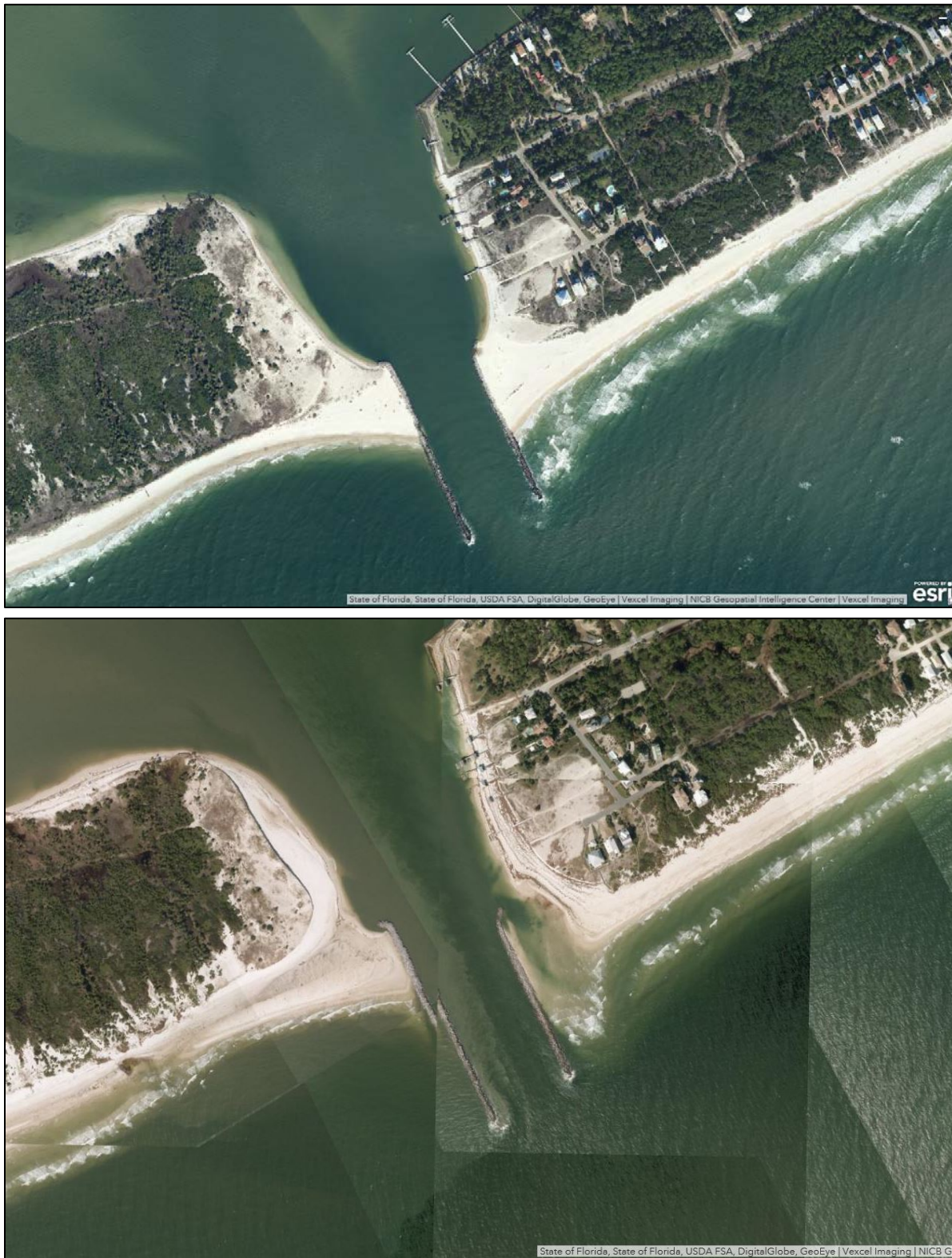
Figure 81. Before (above) and after (below) aerial photos showing breaching of the Bob Sikes Cut jetties from St. George Island, R51-R52. Source: Vexcel Imaging/ NICB Geospatial Intelligence Center.
