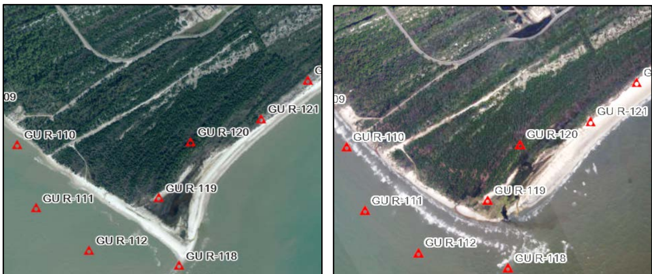
Figure 53. Before and after aerial photos of Cape San Blas showing the loss of 660 feet off the cape at R118. (Source: Vexcel Imaging/ NICB Geospatial Intelligence Center)
