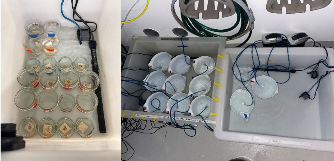
Figure 31 Example of experimental set up. Jars containing larvae for survival trails (left) and holding bowls containing motile larvae for competency trials (right).
