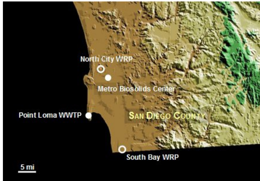
Figure 5-8. Satellite Water Reclamation Systems in San Diego County, California (City of San Diego undated-b; City of San Diego undated-e; City of San Diego undated-c; City of San Diego undated-a). Open points denote satellite facilities and solid points represent regional treatment plants. Facility locations are shown on a digital relief map of California (USGS 2002).
