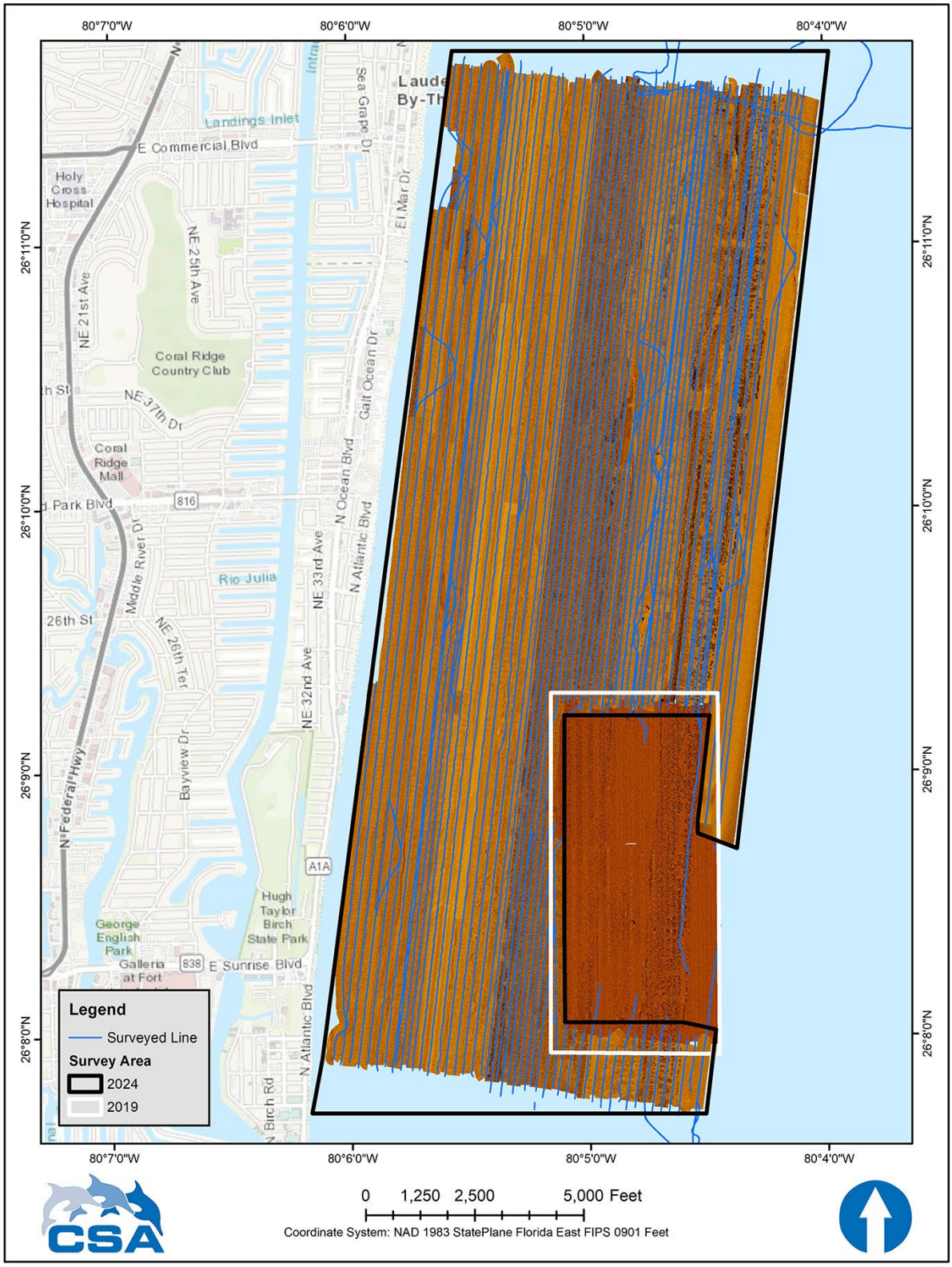
Figure 10. The Osborne Tire Reef 2024 Survey lines overlaid onto the side-scan sonar mosaic data.
