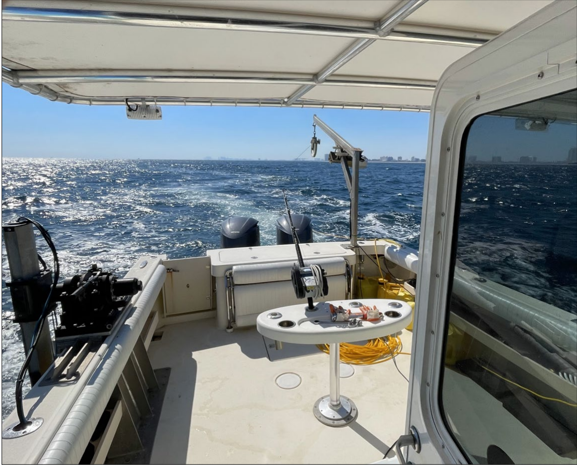
Image 1. Side-scan sonar deployed over the stern of the survey vessel with a davit and sheave block. Multibeam echosounder system on the side pole mounted on the starboard rail in the deployed position.
