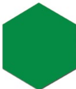
No. 2 Fuel Oil Fill Cover
