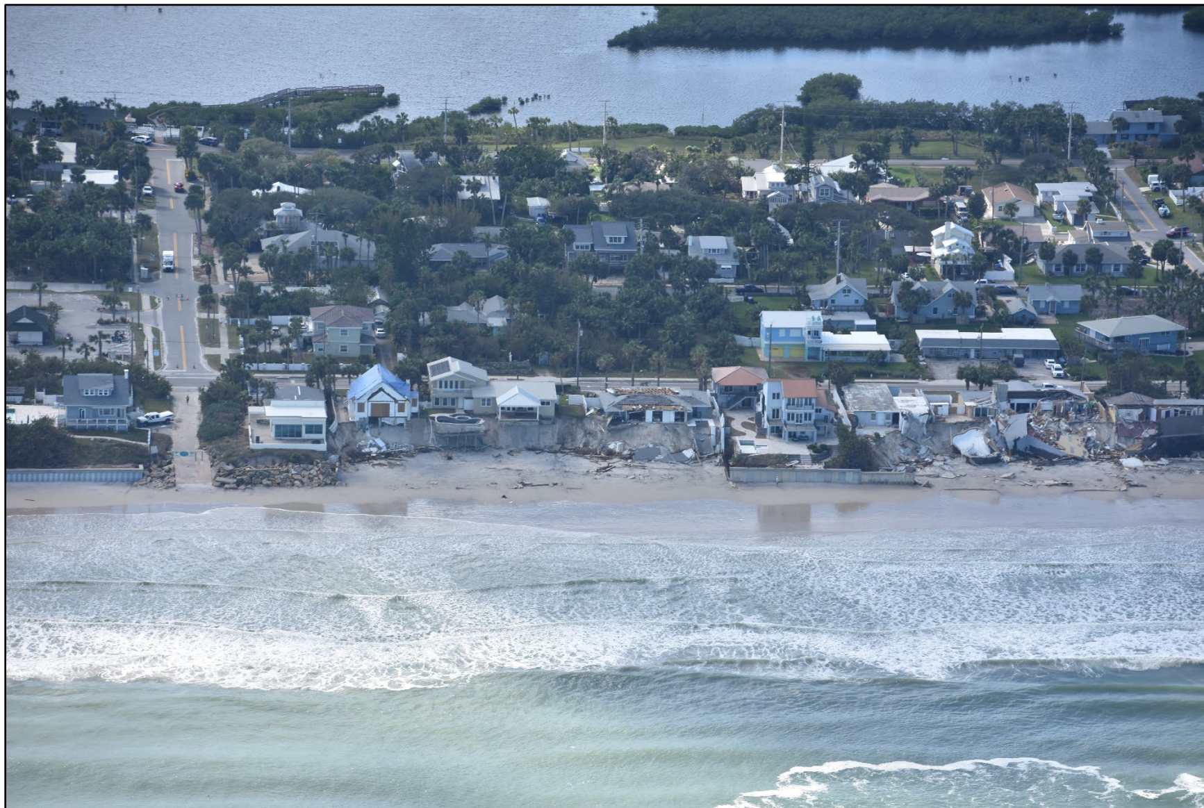
Figure 86. Major erosion damages to seawalls and upland properties at Toronita Avenue in Wilbur by the Sea (R-125). [Credit: Oblique aerial photo by the Civil Air Patrol, November 12, 2022.]
