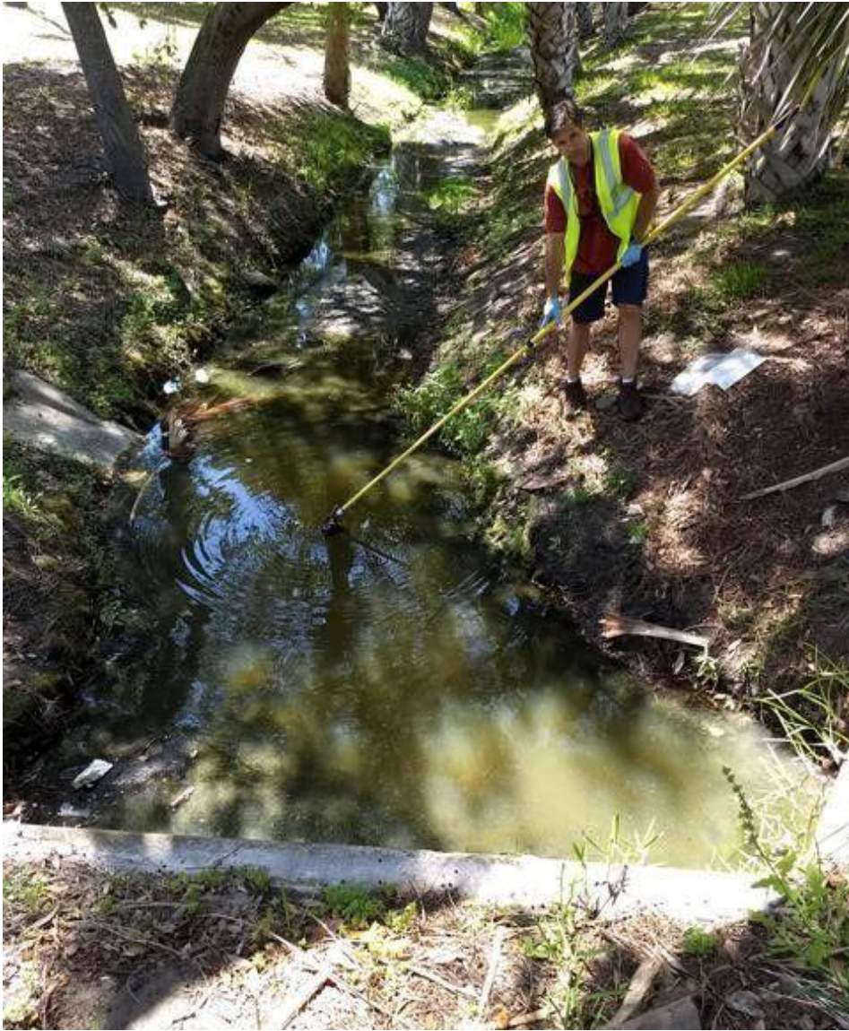
Sampling through a storm grate using a peristaltic pump.
