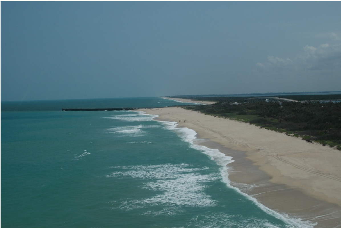
Figure 5. This photo of the Sebastian Inlet (2005) illustrates how inlets can impede the natural flow of sand along the littoral zone and shows the offset of the coastline on either side of the inlet. DEP project file photo.
