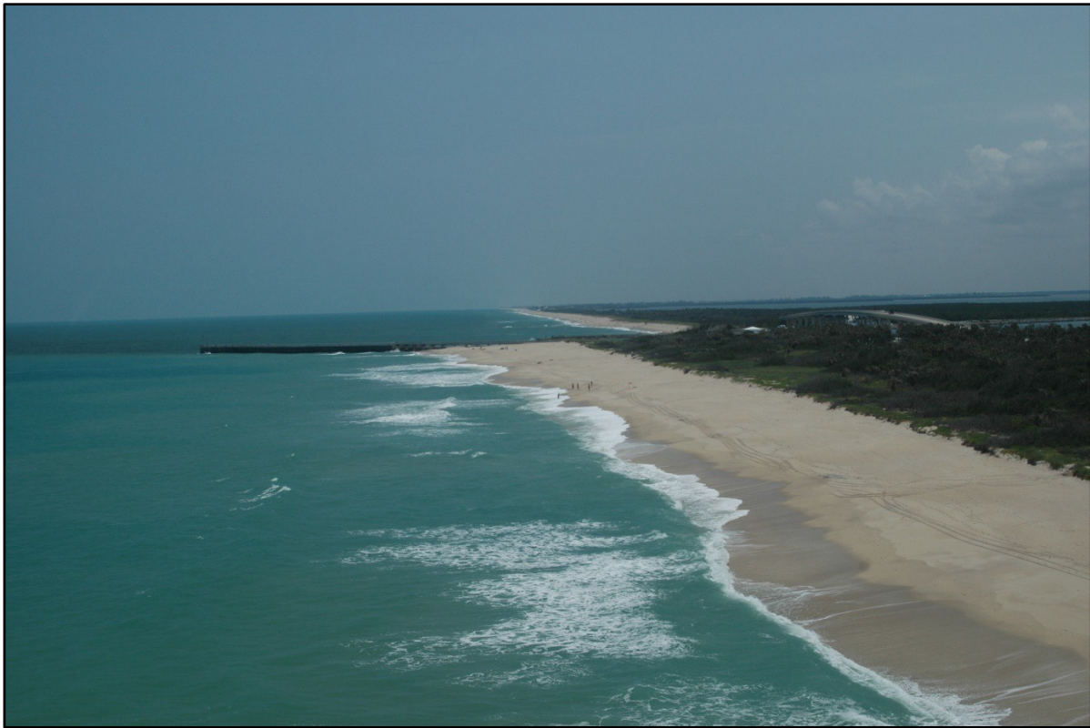
Figure 5. This photo of the Sebastian Inlet from 2005 illustrates how inlets can impede the natural flow of sand along the littoral zone and shows the offset of the coastline on either side of the inlet. DEP project file photo.
