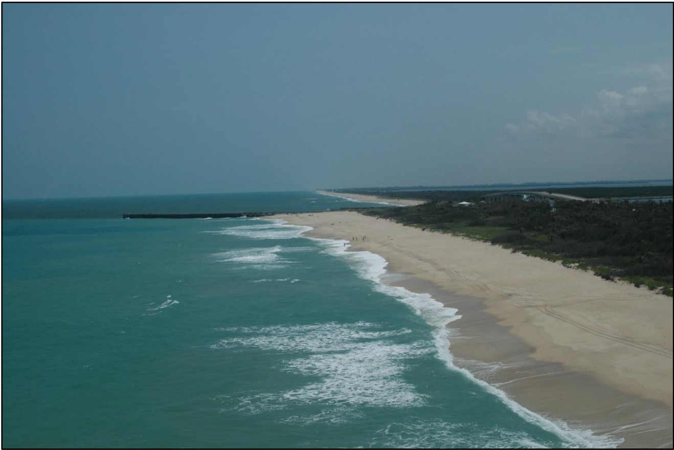
Figure 11. This aerial photo of Sebastian Inlet from 2005 illustrates how inlets can impede the natural flow of sand along the littoral zone and shows the offset of the coastline on either side of the inlet. The offset is common with altered inlets. DEP project file photo.
