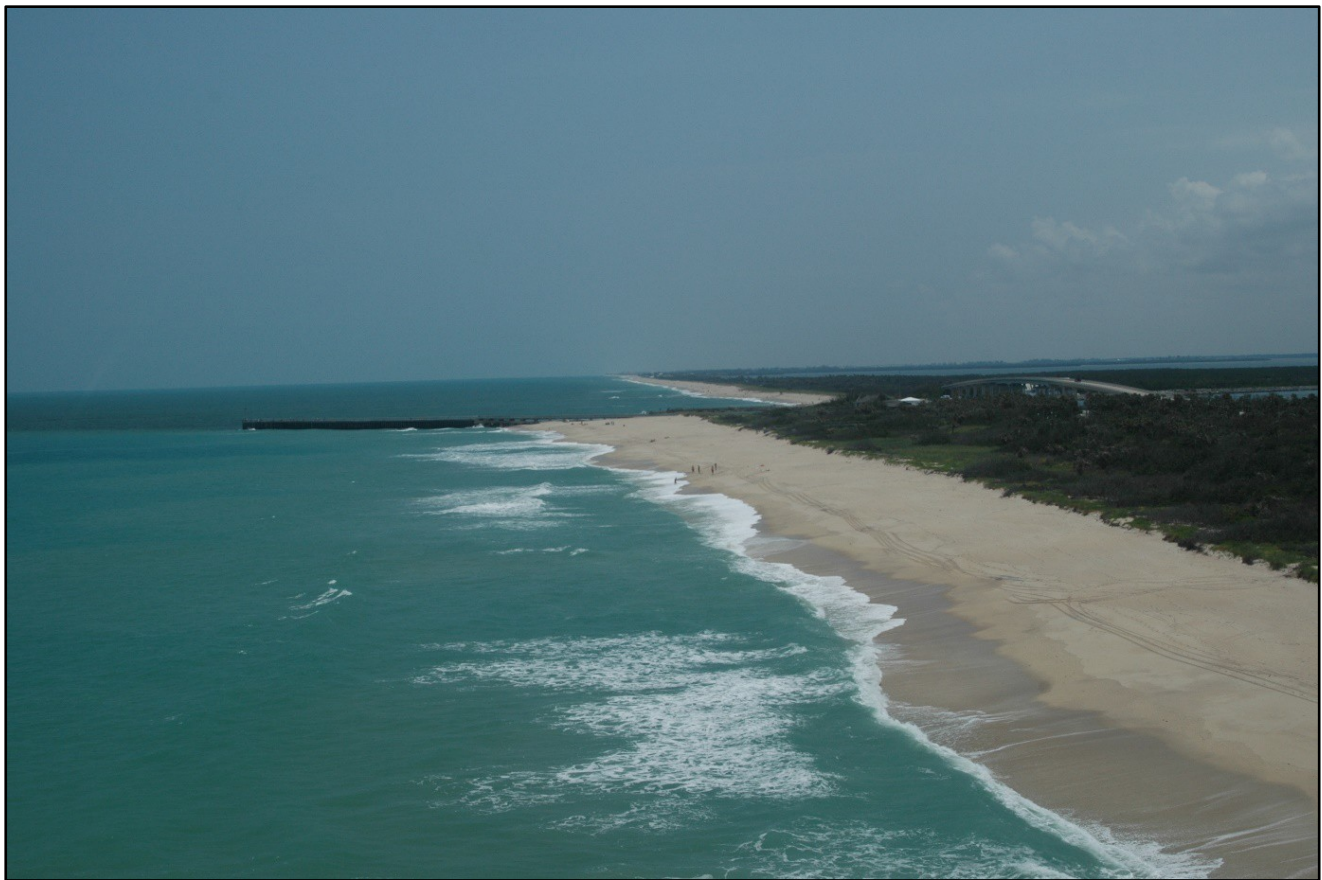
Figure 10. This photo of the Sebastian Inlet from 2005 illustrates how inlets can impede the natural flow of sand along the littoral zone and shows the offset of the coastline on either side of the inlet. DEP project file photo.
