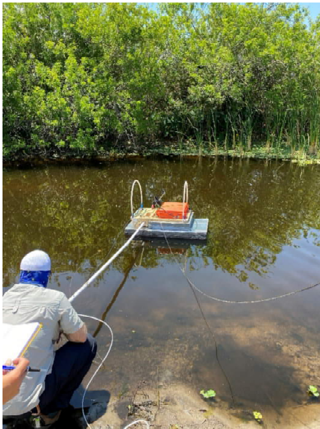
Figure 1. Lake sampling device collecting water samples and spectral data. Figure 2. Collecting WS-066 and spectral data and spectral data.
