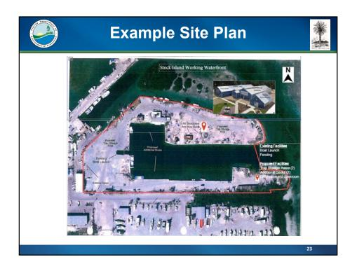
**Exhibit Y – Conceptual Site Plan** – Make sure your site plan clearly delineates the Project Boundaries and shows the approximate location of all proposed site improvements. Make sure you address all existing facilities, renovation of existing facilities and any new facilities. Also make sure you label everything as existing, renovation and new. Also include:
