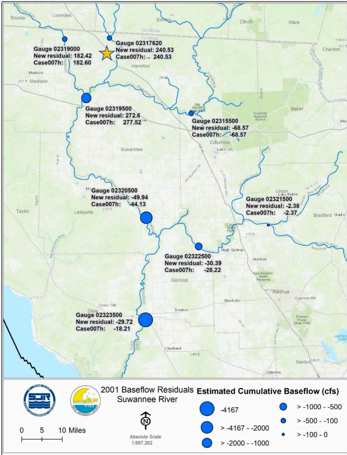
Figure 7: Comparison of Cumulative Baseflow Rate Residuals for Select USGS Gauges, 2001. NSFEG.V.1.1 Addendum Page 38.
