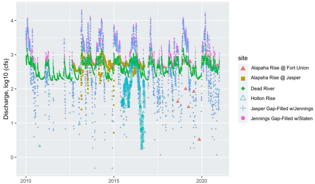
Figure 25: Reconstructed Discharge for Flow Stations Above and Below Swallets, and Reconstructed Dead River Flows. 2010 - 2020. Data Displayed in Log Scale.
