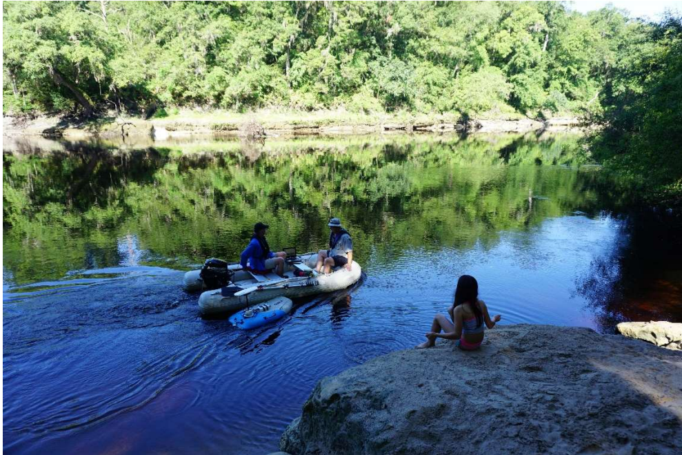
Figure 5: ADCP data collection setup showing motorized zodiac with ADCP w/GPS deployed on a small float.
