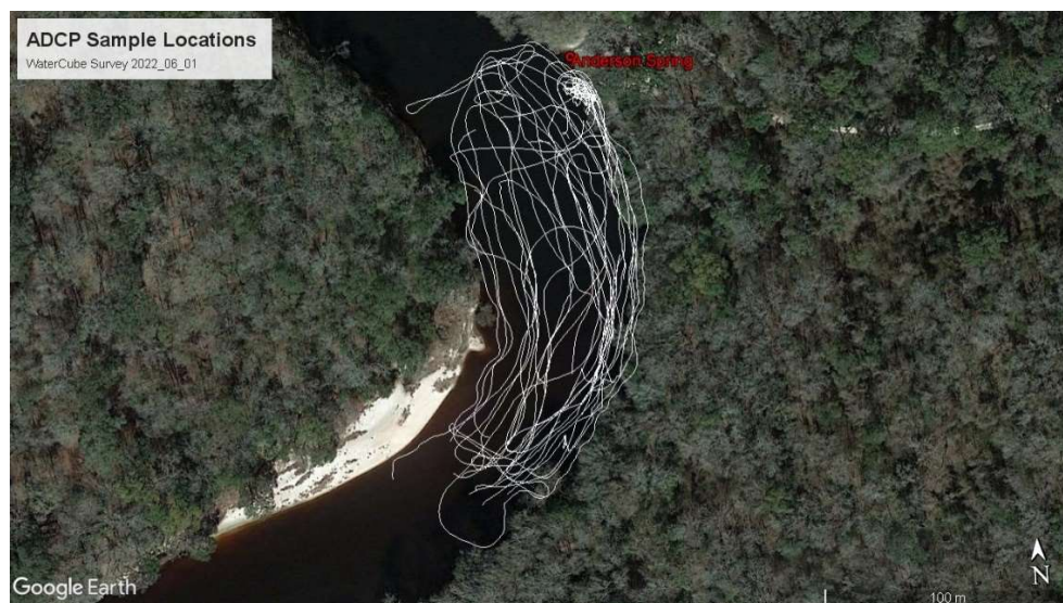
Figure 6: ADCP data collection track lines for Anderson Springs WaterCube survey June 1st, 2022.
