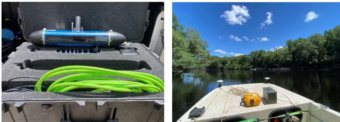
Figure 2: Ping DSP 3DSS Sonar Array (left) and RTK GPS (left) used on SRWMD survey vessel.
