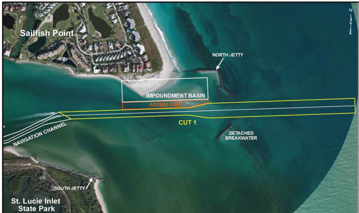
Figure 3. Authorized federal navigation channel, sediment impoundment basin, jetties and breakwater (Kremkau et al, 2013).
