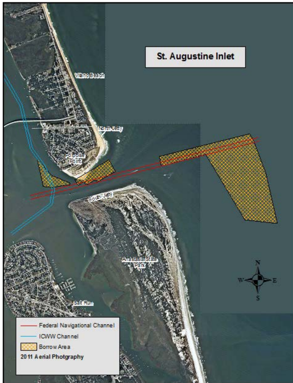
Figure 2. St. Augustine Inlet with Federal Project Dredging Areas
