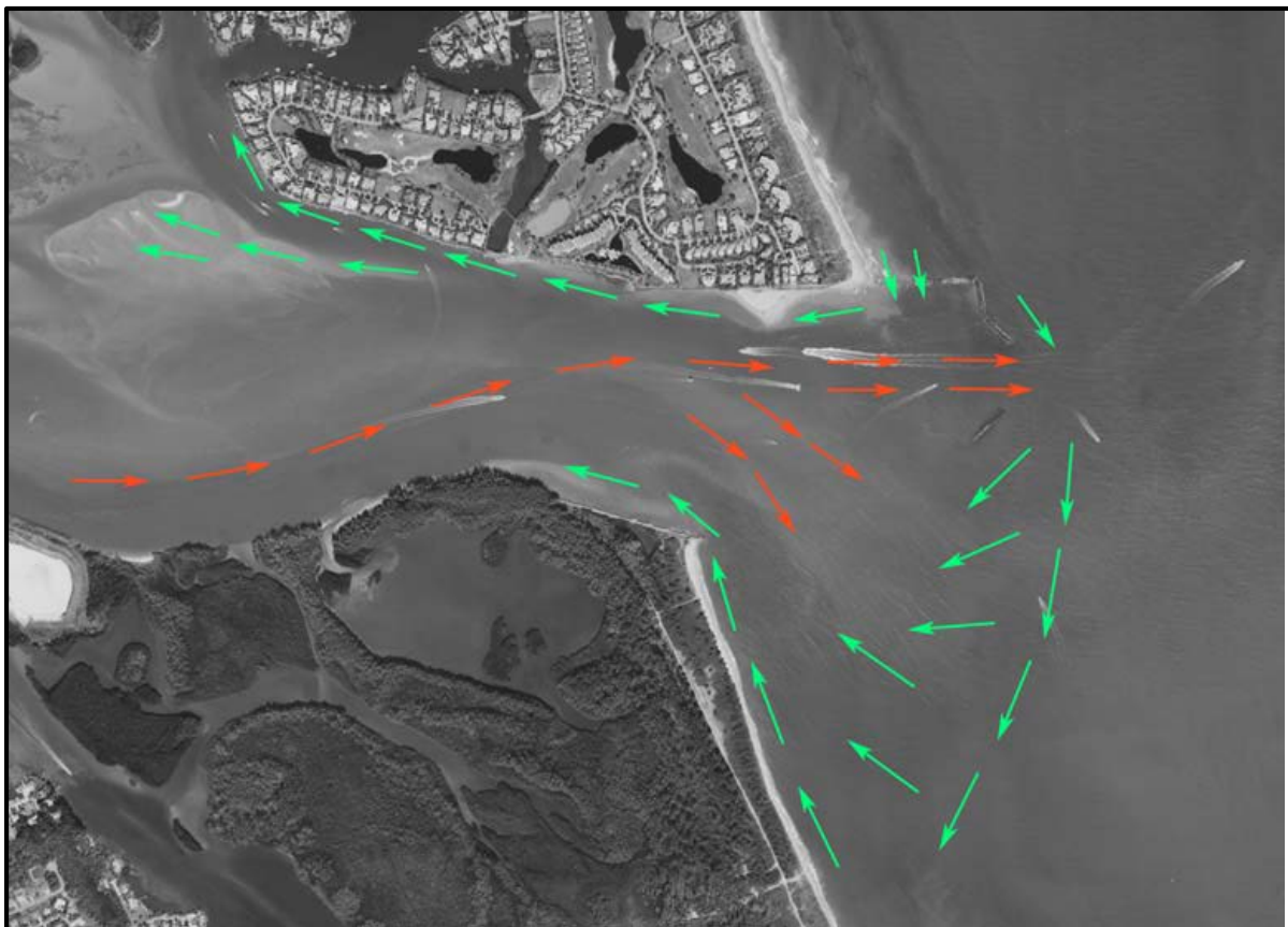
Figure 5. General flood and ebb sediment transport pathways (Ramsey et al, 2006).
