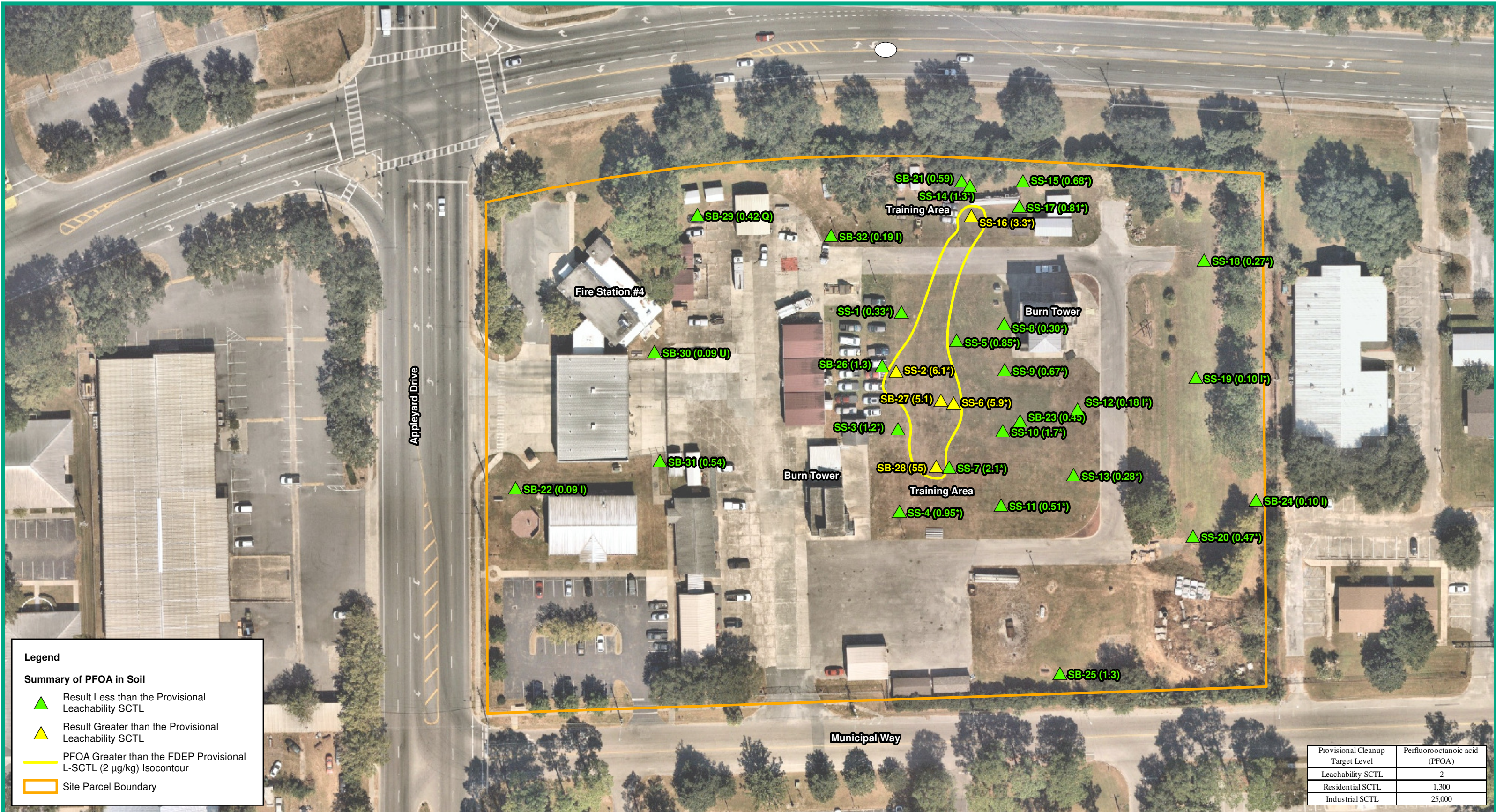
Figure 11B Summary of PFOA in Soil from 0 to 0.5 ft BLS Tallahassee Fire Department 2964 Municipal Way Tallahassee, Leon County, Florida FDEP Facility NO. ERIC_7413
