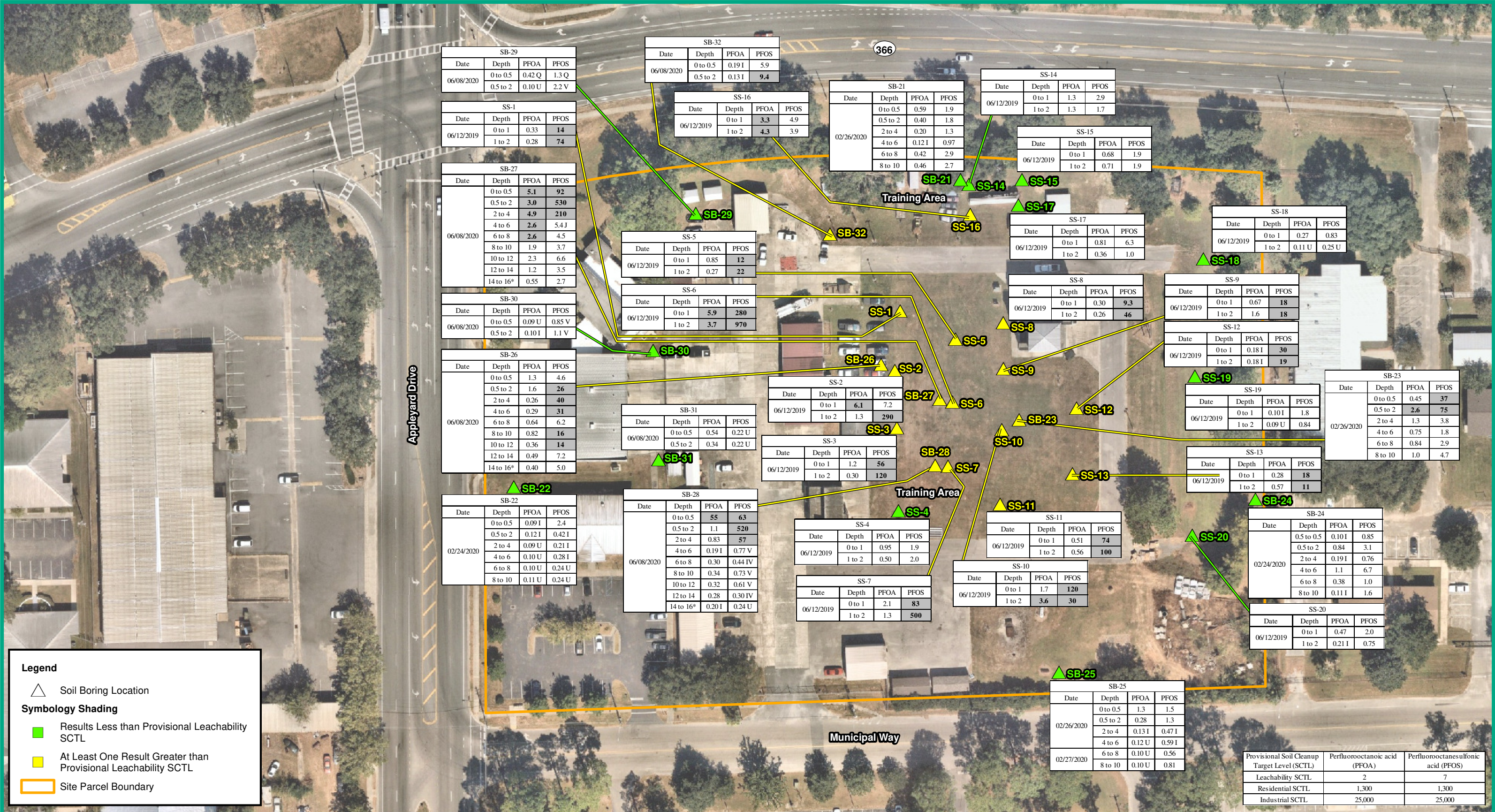
Figure 10 Summary of Analytical Results in Soil Tallahassee Fire Department 2964 Municipal Way Tallahassee, Leon County, Florida FDEP Facility NO. ERIC_7413
