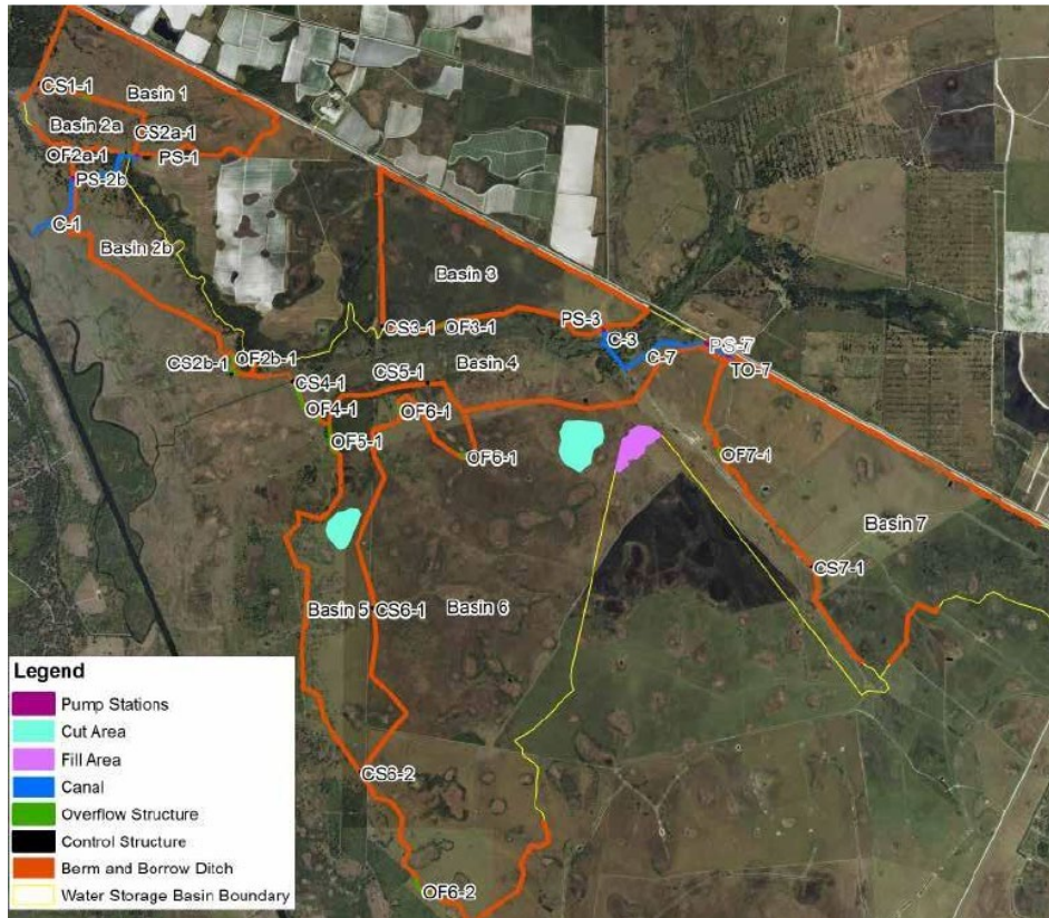
Figure 18. Layout of El Maximo Ranch project basins, berms, control structure, overflow structure, pump stations (Higgins Engineering, 2020)
