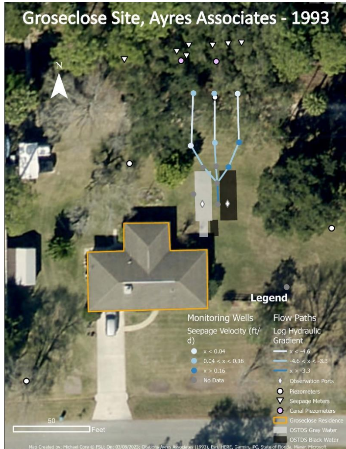
Fig. 16. Diagram shows the pairs of hydraulic heads used for estimating hydraulic gradients. Hydraulic heads and a survey of the Groseclose house and its drainfield locations were given by Ayres Associates (1993).
