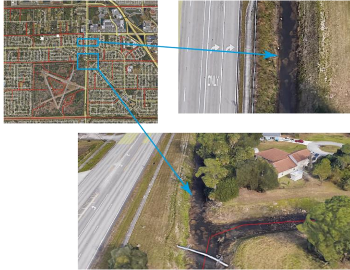
Fig. 2.7. Canals on the east side of Minton Road shown on Google Earth but not in NHD data downloaded from FGDL website.
