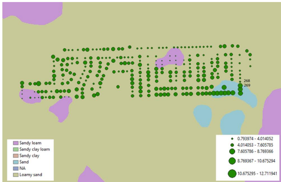
Fig. 2.30. VZMOD-simulated \text{NO}_3\text{-N} concentrations around the Groseclose and Jones homes.
