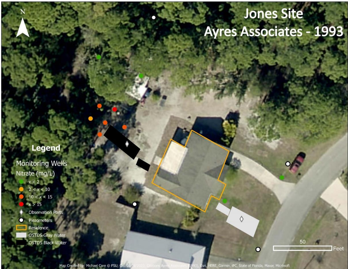
Fig 5.11. Map of the Jones Site, Turkey Creek, with nitrate levels from Ayres Associates (1993). The map of the Jones property shows the residents in an orange outline and the monitoring well locations in green, orange, and red dots based on nitrate concentrations.
