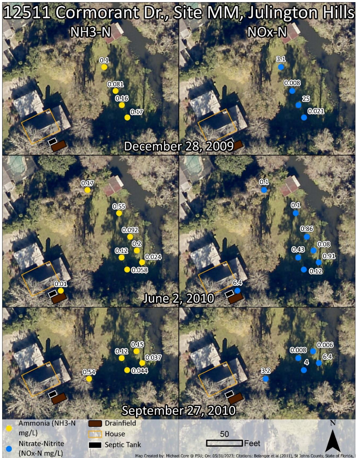
Fig. 5.19. Map of Julington Heights, MM locations for BN. The maps show the MM site with the septic tank marked as a black rectangle, the drainfield marked as a brown rectangle, and the monitoring wells in blue and yellow dots.
