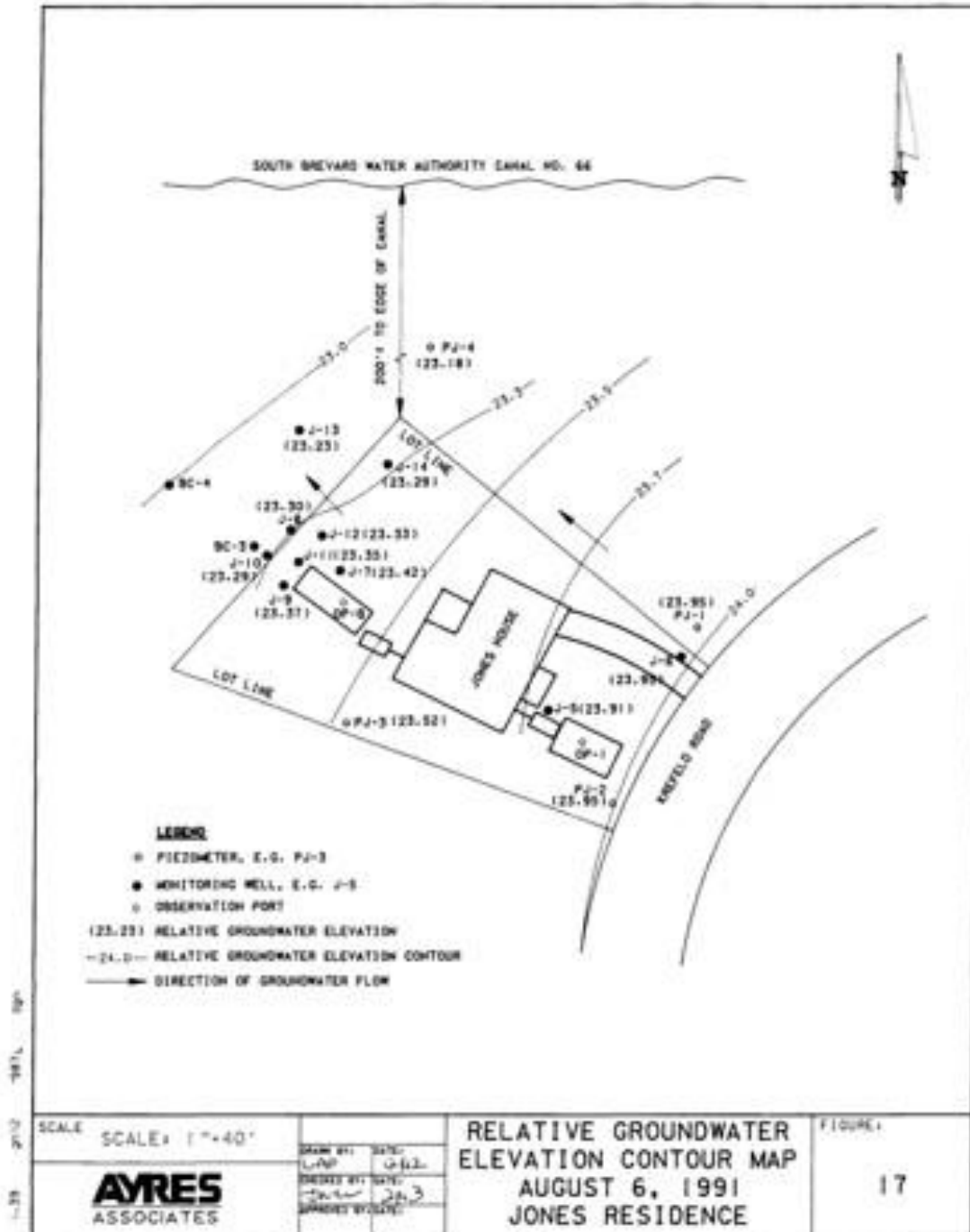
Fig. 5.4. Groundwater flow direction at the Jones Site, Turkey Creek, Ayres Associates (1993). The boundary survey shows the Jones residents in a black outline and the groundwater elevation in black contour lines.
