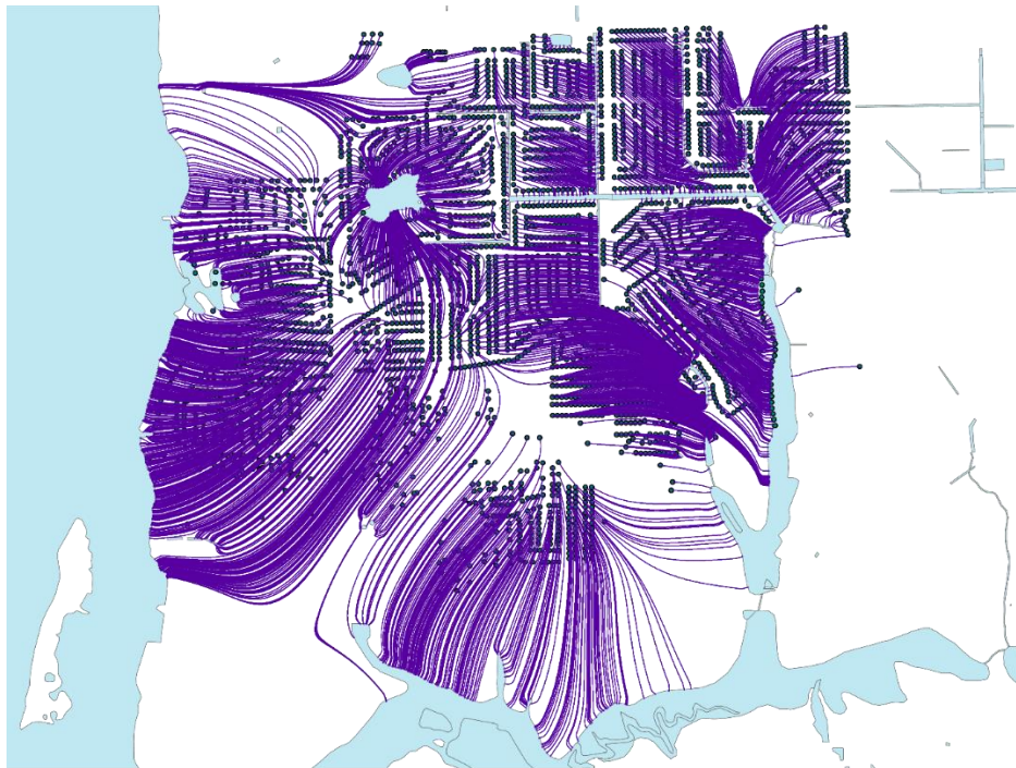
Fig. 4.4. Simulated flow paths from septic tanks to surface water bodies of Eggleston Heights.
