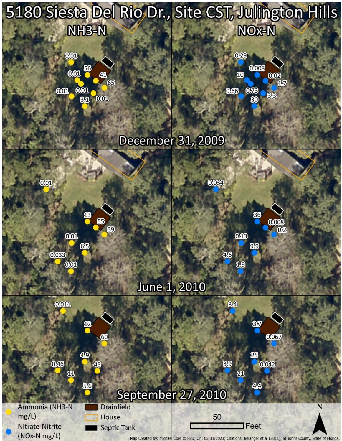
Fig. 5.17. Map of Julington Heights, CST locations for BN. The maps show the CST site with the septic tank marked as a black rectangle, the drainfield marked as a brown rectangle, and the monitoring wells in blue and yellow dots.
