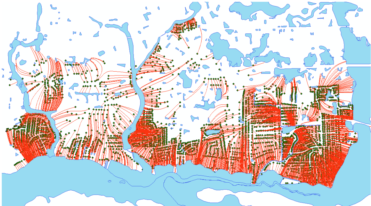
Fig. 4.20. Simulated flow paths from septic tanks to surface water bodies of Julington Creek.
