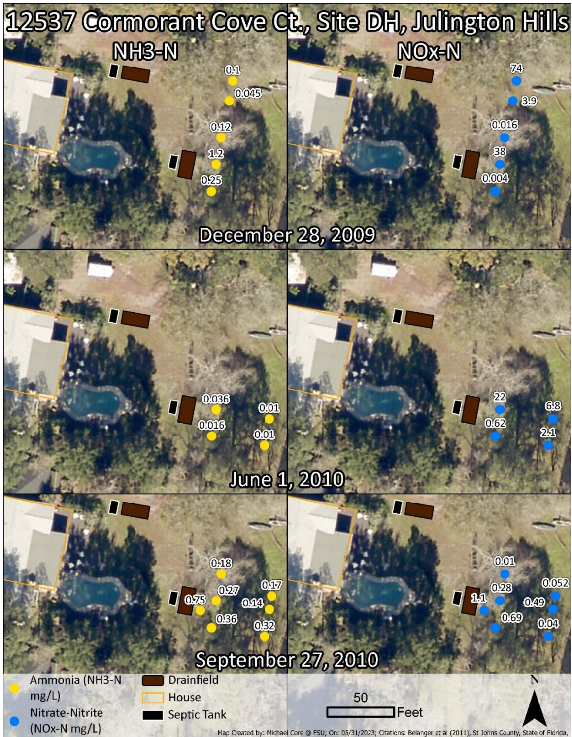
Fig. 5.18. Map of Julington Heights, DH locations for BN. The maps show the DH site with the septic tank marked as a black rectangle, the drainfield marked as a brown rectangle, and the monitoring wells in blue and yellow dots.
