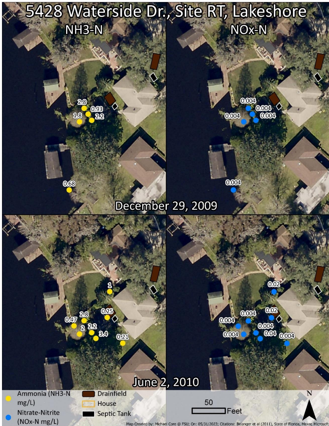
Fig. 5.20. Map of Lakeshore, RT locations for BN. The maps show the MM site with the septic tank marked as a black rectangle, the drainfield marked as a brown rectangle, and the monitoring wells in blue and yellow dots.
