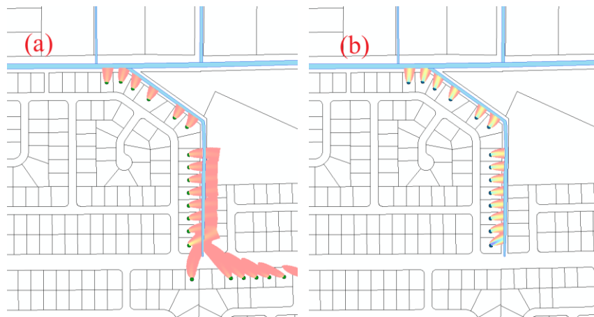
Fig. 2.38. Nitrogen plumes for two situations: (a) OSTDS are located on both sides of canal, and (b) OSTDS on only one side of canal.
