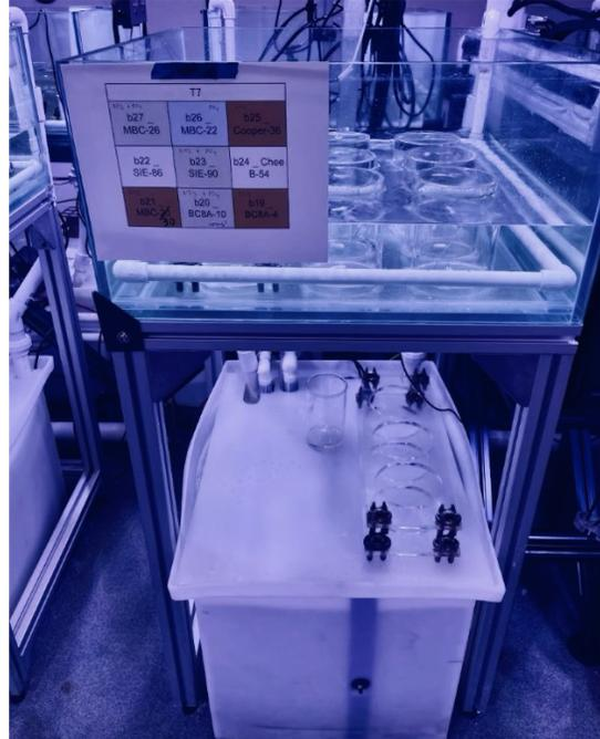
**Figure 4:** Changes performed in the tank stands to allow more stability in the arm system. **A.** Assembled aluminum stands for the new systems. **B.** Aluminum stands installed in the Experimental Reef Lab holding a glass tank, the new stir plates and the new coral vessels.
