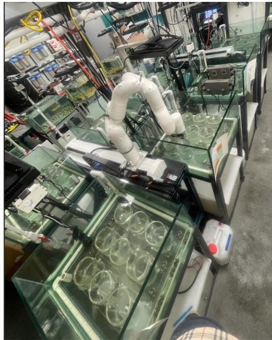
**Figure 7:** Modified STAR system running without corals to test the stability of the dosing system.
