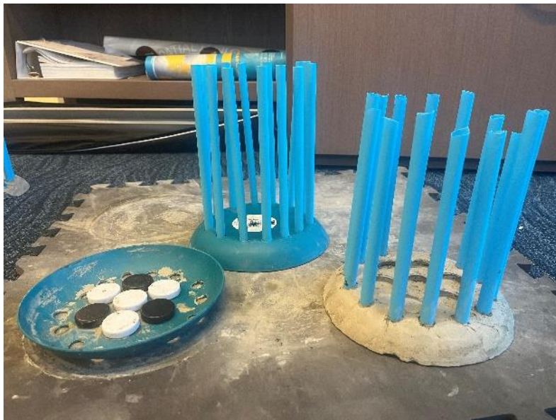
Figure 20. Process of creating cement domes fitted with PHA straws.
