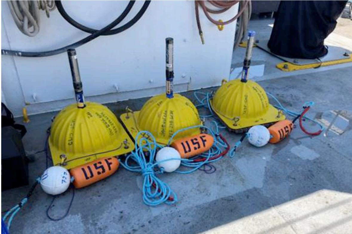
**Figure Weisberg-5.** Images of the three water quality bottom mounts.
