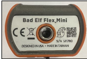
Figure 3. Bad Elf 2500 GNSS Unit bottom with ¼" x 20 thread mount.
