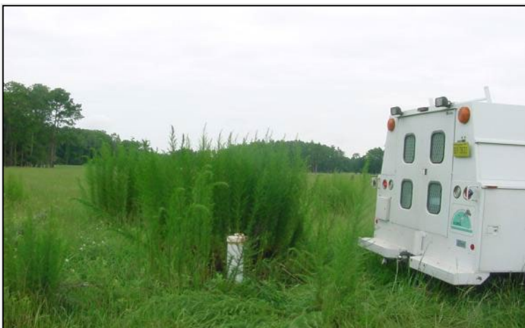
Figure 40. Example of hidden well. This well is in a stand of grasses.
