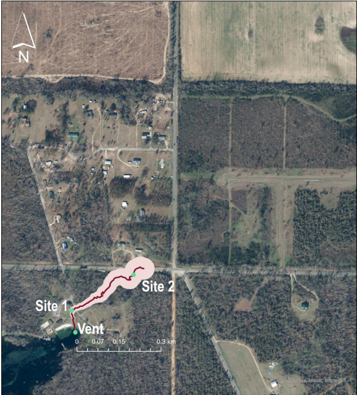
Figure 19: The mapped conduit (red line) and horizontal error (shaded pink) associated with increasing penetration.
