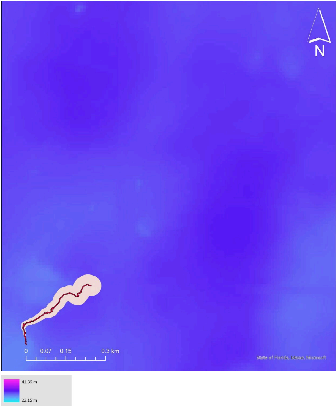
Figure 20: DEM and mapped conduit (red line) and horizontal error (shaded pink) associated with increasing penetration. The DEM was obtained from USGS National Map Viewer ( https://www.usgs.gov/programs/national-geospatial-program/national-map ) DEM, satellite, and land use are within the same window.
