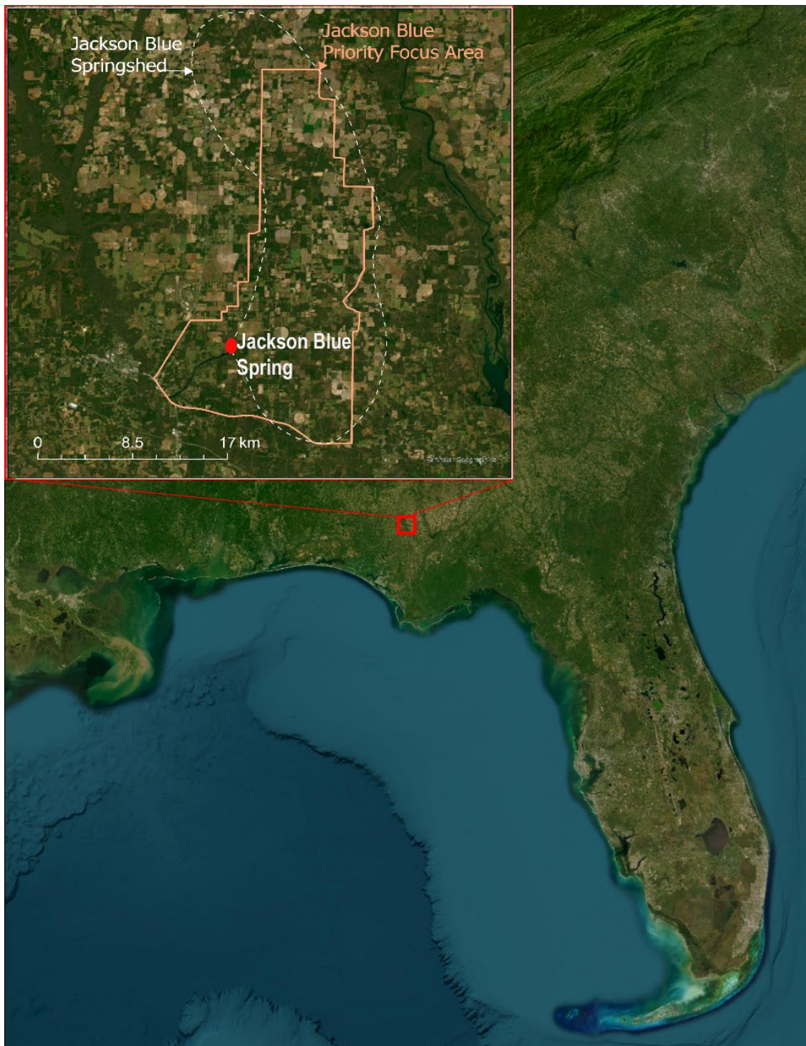
Figure 5: Location of Jackson Blue Spring area in the Dougherty Karst Plain and eastern panhandle. Both the springshed identified from topographic maps and later refined through potentiometric surface contours is shown as white dashed line. The priority spring area is shown as a solid orange line.
