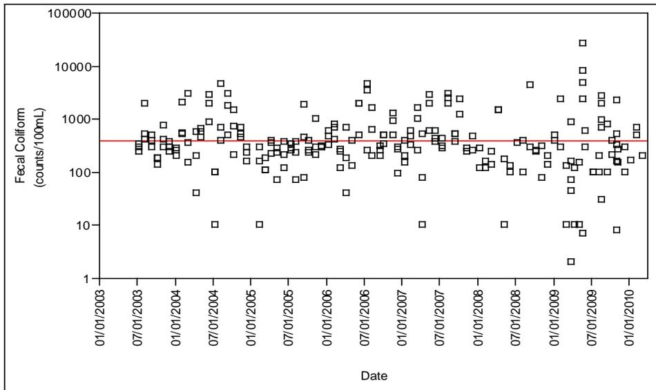
Figure 5.2d. Fecal Coliform Concentrations Over Time in the C-6 (Miami River) Lower Segment (WBID 3288B) During the Cycle 2 Verified Period (January 1, 2003–June 30, 2010)
