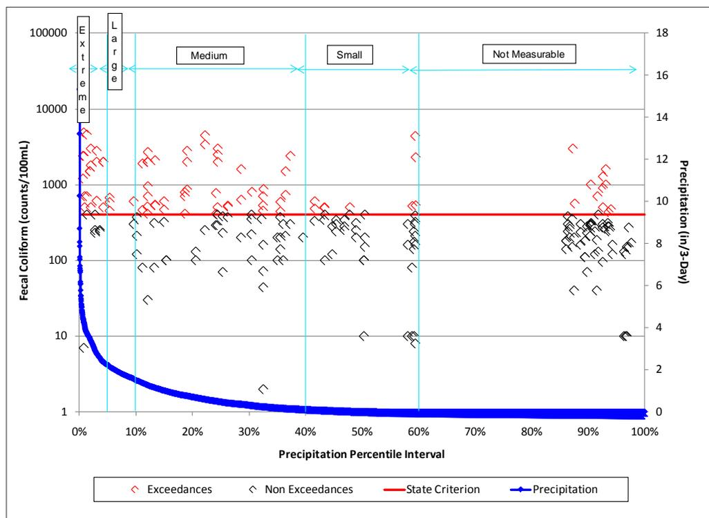
Figure 5.7d. Fecal Coliform Data During the Cycle 2 Verified Period (January 1, 2003–June 30, 2010) by Hydrologic Condition for the C-6 (Miami River) Lower Segment (WBID 3288B)
