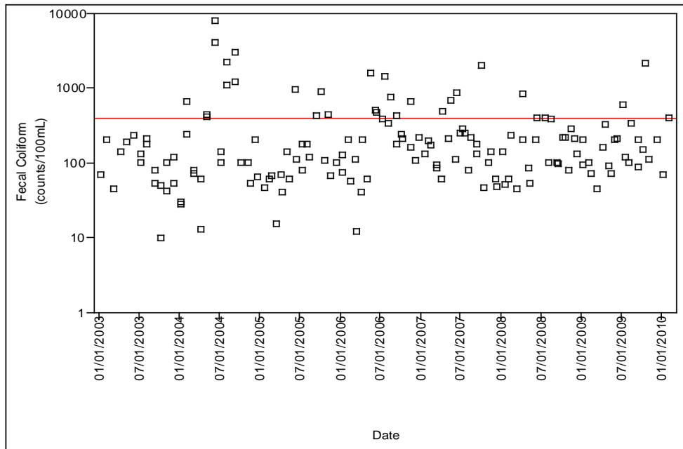
Figure 5.2e. Fecal Coliform Concentrations Over Time in the C-6 (Miami) Canal (WBID 3290) During the Cycle 2 Verified Period (January 1, 2003–June 30, 2010)
