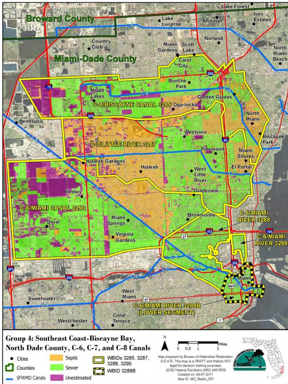
Figure C.1. Distribution of Onsite Sewage Disposal Systems (Septic Tanks) within the Boundaries of WBIDs 3285, 3287, 3288, 3288B, and 3290
