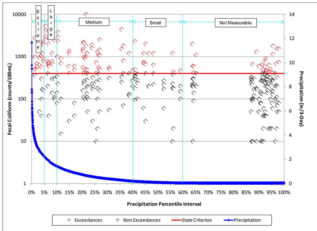
Figure 5.7b. Fecal Coliform Data During the Cycle 2 Verified Period (January 1, 2003–June 30, 2010) by Hydrologic Condition for the C-7 (Little River) Canal (WBID 3287)
