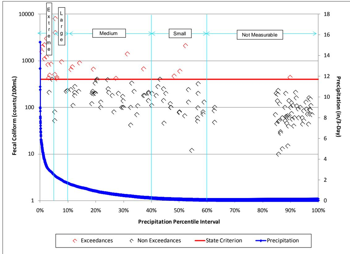
Figure 5.7e. Fecal Coliform Data During the Cycle 2 Verified Period (January 1, 2003–June 30, 2010) by Hydrologic Condition for the C-6 (Miami) Canal (WBID 3290)
