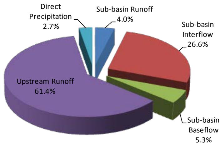
Figure 5.13. Percent TP Contribution to Lake Jackson under the Existing Condition During the Simulation Period, 2000–06
