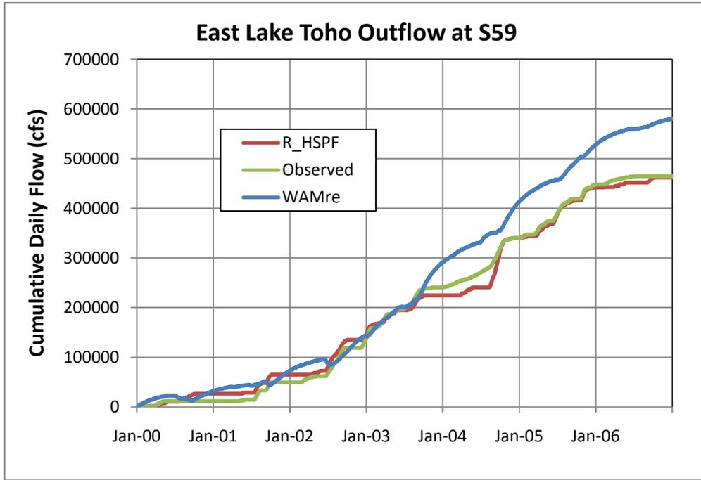
Figure D-13. Observed Versus Simulated Cumulative Daily Flows for East Lake
