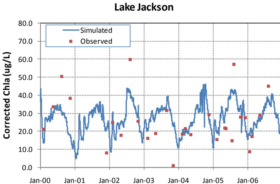
**Figure 5.22. Time-Series of Observed Versus Simulated Daily CChla Concentrations in Lake Jackson During the Simulation Period, 2000–06**
