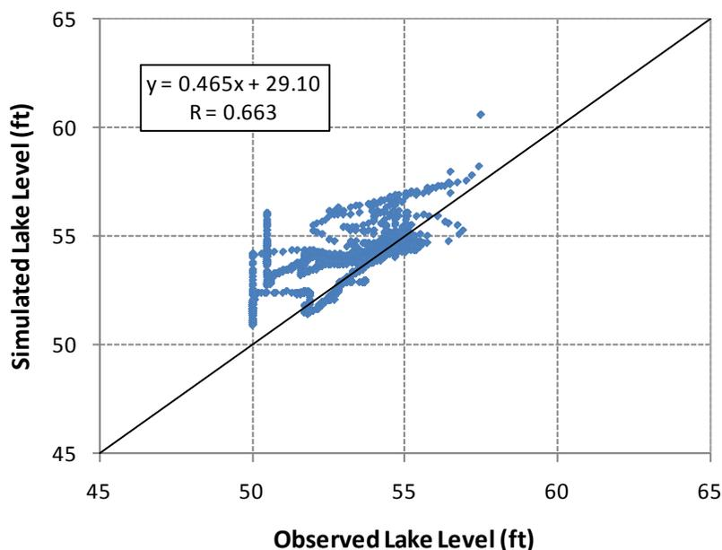
**Figure 5.9.** Daily Point-to-Point Paired Calibration on Lake Level (feet) During the Simulation Period, 2000–06 (solid line indicates the ideal 1-to-1 line, R represents a correlation coefficient of the best fit between observed and simulated lake levels, and n indicates the number of observations)
