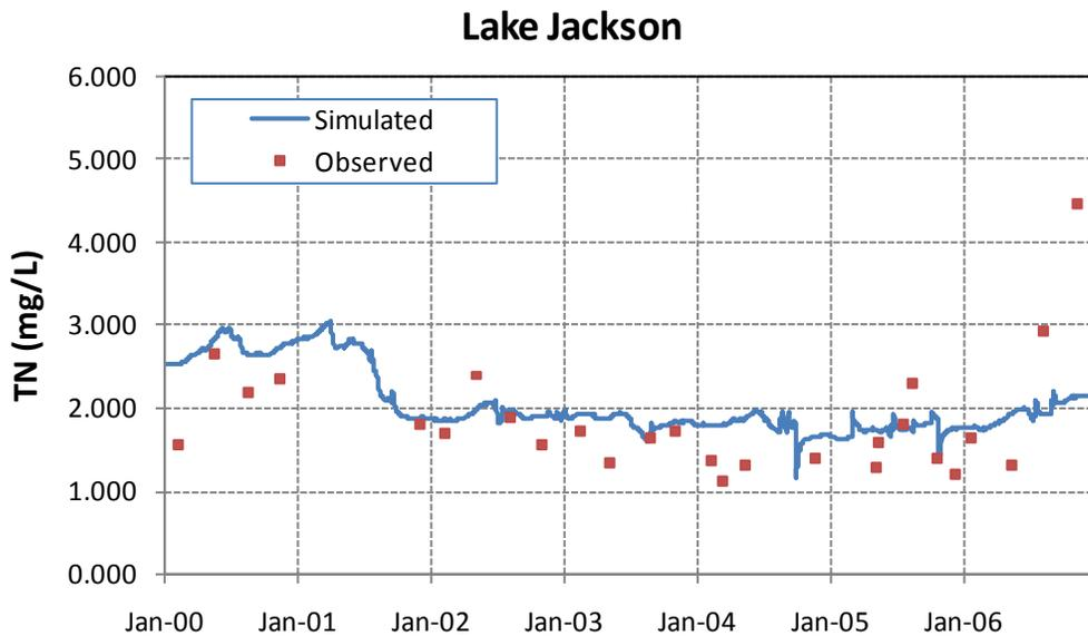
Figure 5.16. Time-Series of Observed Versus Simulated Daily TN Concentrations in Lake Jackson During the Simulation Period, 2000–06
