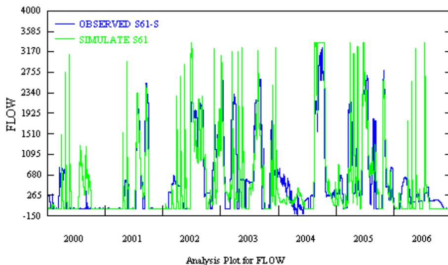
**Figure D-4. Observed Versus Simulated Daily Flow (cfs) at S61 for Lake Tohopekaliga Outflow, 2000–06**
