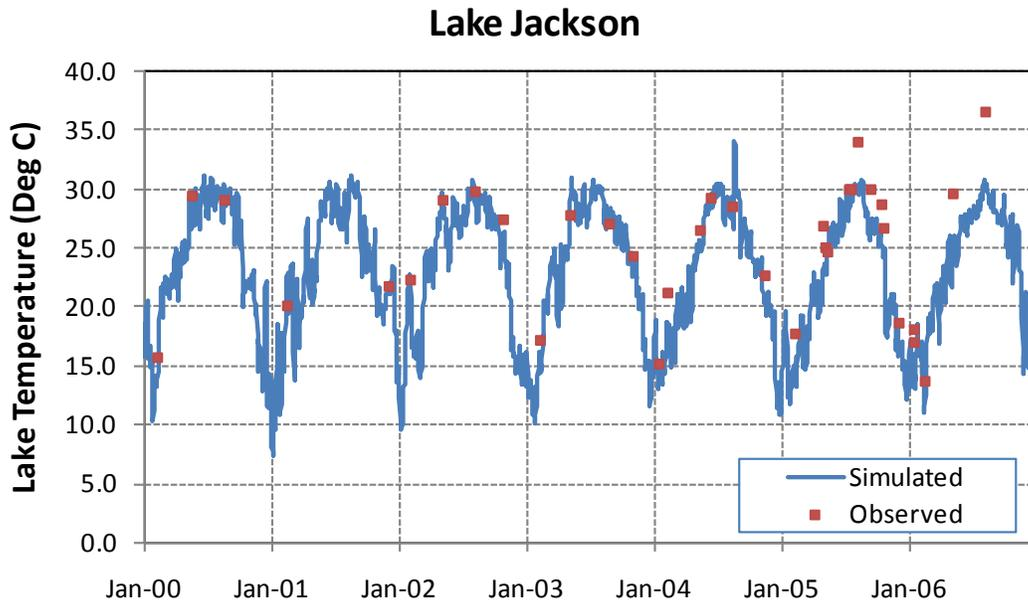
Figure 5.5. Observed Versus Simulated Daily Lake Temperature (°C.) in Lake Jackson During the Simulation Period, 2000–06
