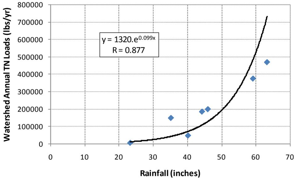
**Figure 5.14. Relationship between Rainfall Versus Watershed Annual TN Loads to Lake Jackson under the Existing Condition During the Simulation Period, 2000–06**
