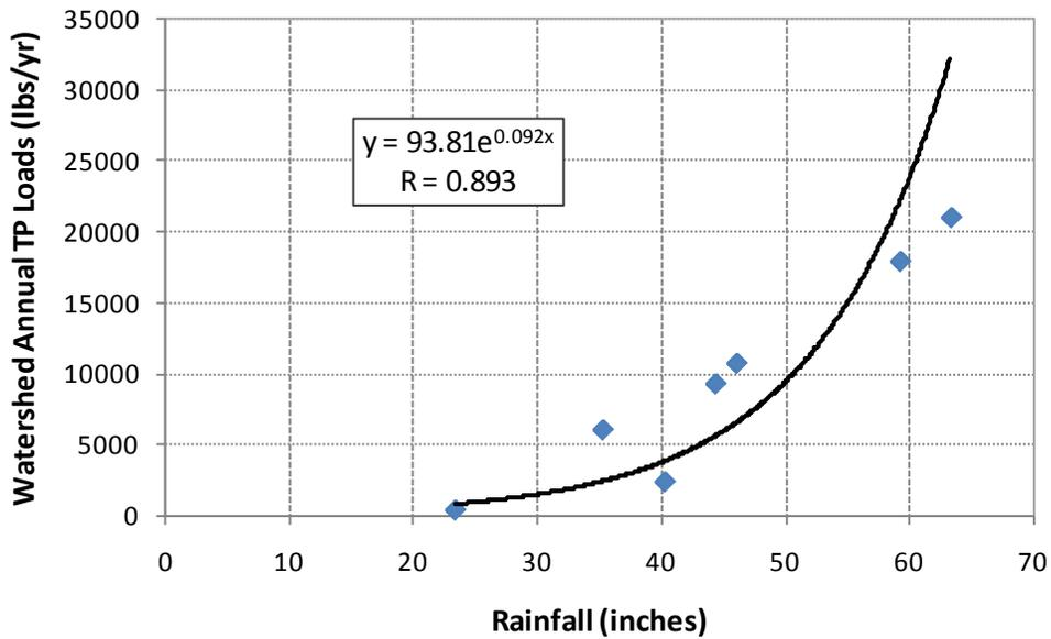
**Figure 5.15. Relationship Between Rainfall Versus Watershed Annual TP Loads to Lake Jackson under the Existing Condition During the Simulation Period, 2000–06**
