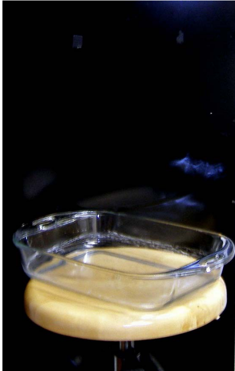
Figure 3: Pyrex baking dish for drying collected sample (clean and dry before pouring in sample)
