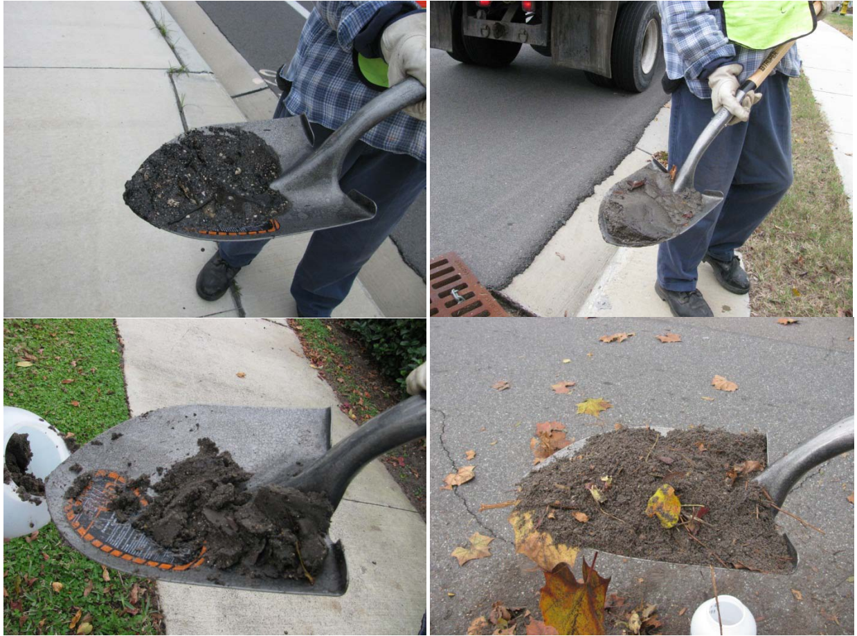
Figure 1: Visual indication of moisture content variability that can be observed in collected samples of solids that have been recovered during the MS4 study (can vary from dry to wet (top left))
