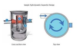
all primarily rely on swirl action and particle settling to remove pollutants. They appear to be most effective when used for pretreatment in areas where runoff is expected to contain sediment particles greater than 100 microns in diameter. Types of hydrodynamic separators include Stormceptor, Storm Treat, VortSentry, Continuous Deflection Separator (CDS) and Aqua-Swirl.
