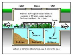
• **Hydrodynamic separators** are small, flow-through devices that remove sediment, trap debris, and separate floating oils from runoff. While their proprietary designs vary, they
